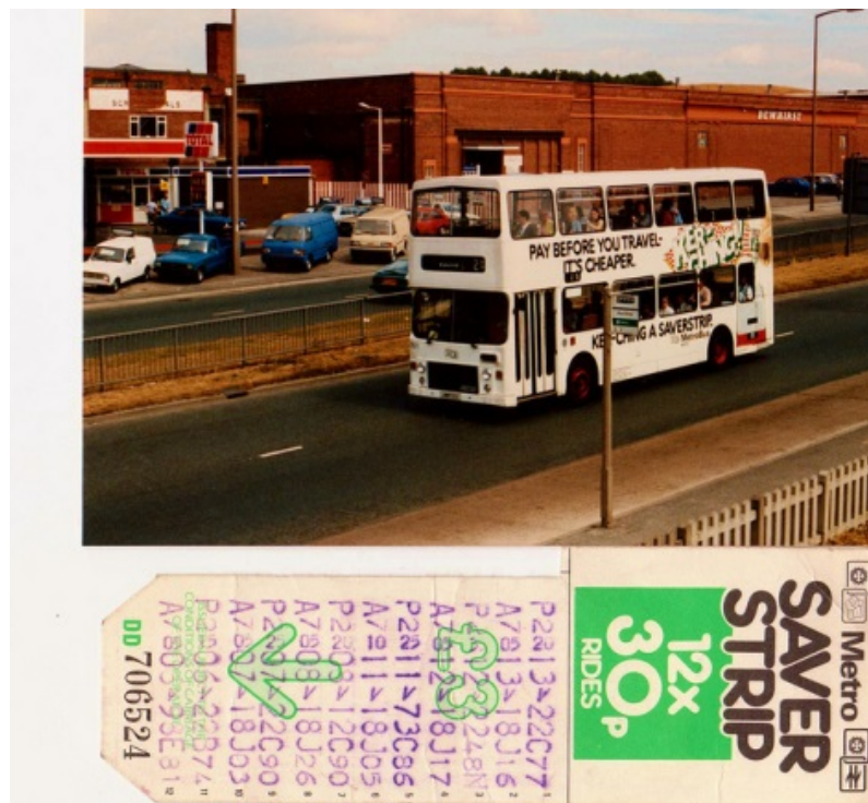
Fig. 3.10 Top: A publicly owned Metrobus travel down the York Road towards the city centre on the eve of deregulation in 1986. Below: a Metro Saver Strip, a multi-use ticket designed to minimise passenger loading time at bus stops and make bus travel more attractive [Clifford Stead, flickr, https://www.flickr.com/photos/cliffordstead/albums , accessed 17 February 2015]
