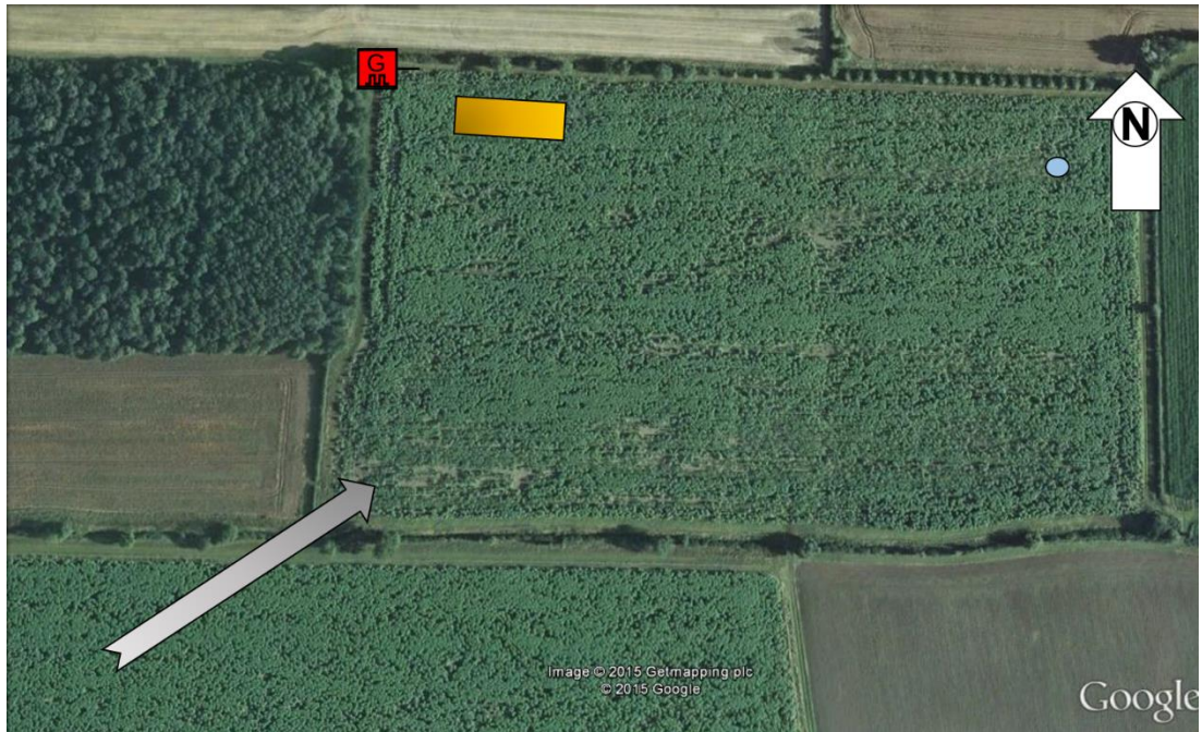
Figure 3.3 Aerial view of experimental site. Arrow marked “N” indicates the direction of North. The prevailing wind direction is denoted by the elongated arrow. The circle in the north-eastern region of the field shows the location of the EC system, and the rectangle in the north-west corner is the SkyBeam system. The square containing “G” symbolises the diesel generator for powering the equipment. The northern half of the western boundary of the Miscanthus field was bordered by a mature deciduous wood, exceeding 10 m in height. The southern half of the western boundary was adjacent to another Miscanthus field, as was the western half of the south boundary. The neighbouring field at the eastern half of the south boundary was dedicated to conventional arable crop rotation (barley and oilseed rape during the experimental period), as were the two fields to the north of the Miscanthus . The entire eastern side of the Miscanthus was bordered by a short rotation coppice stand which was approximately 3 m tall during the study.
