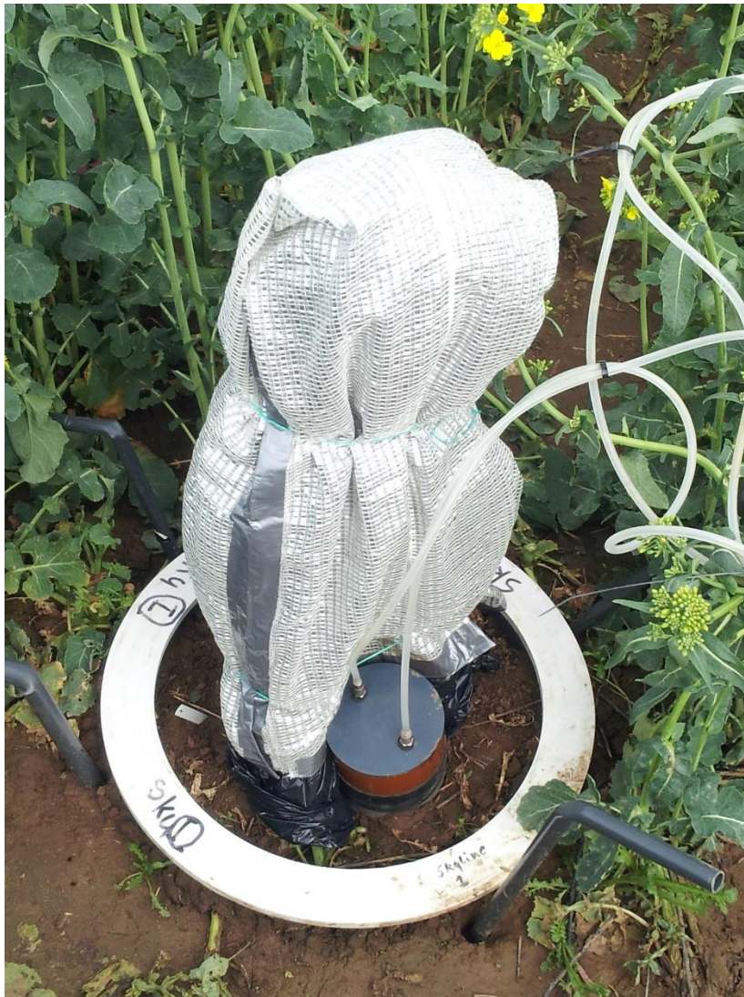
Figure 4.4 Example of a FER ring with shaded vegetation. The shroud did not go all the way to the soil surface in order to allow gas to circulate. Inside the large SkyLine ring is a small opaque chamber, allowing measurement of GHG flux from just the soil.
