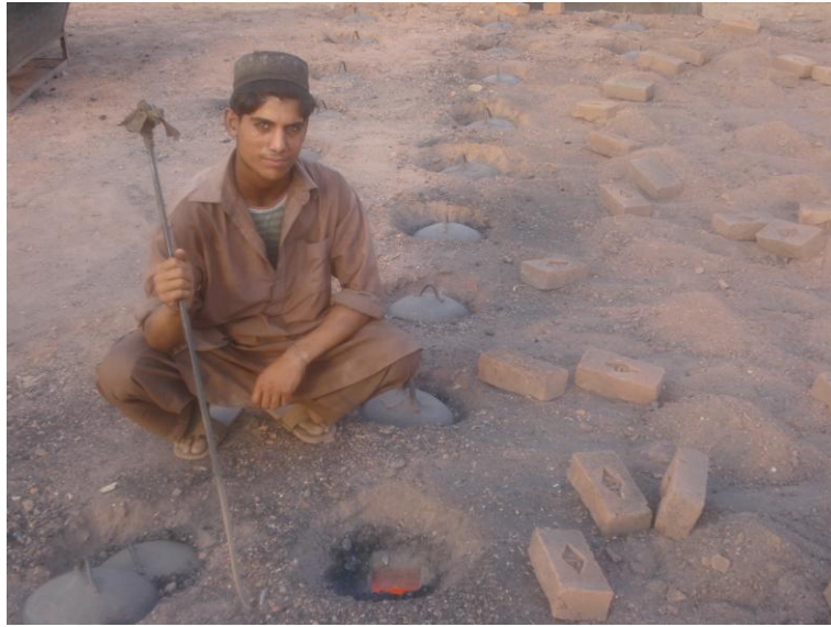
Figure 4.6: A young worker is shown sitting near the fire holes. These have a removable iron lid through which the fuel is dropped in for brick baking.
