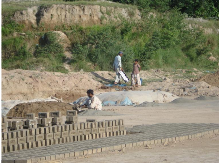
Figure 4.3: Drying the green bricks in the sun before baking near brick kiln factory in Peshawar
