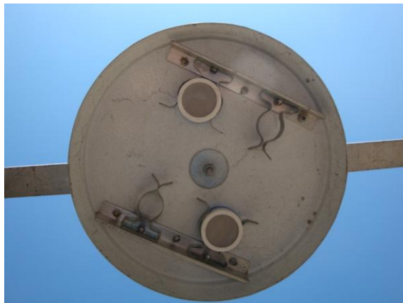
4.8. Inside view of the plate containing passive sampler with the help of hooks at ARI Date 14/12/2008
