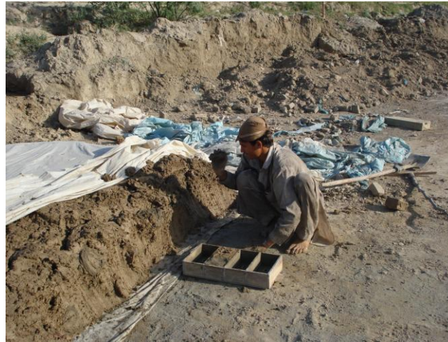
Figure 4.2: A worker preparing green bricks from clay paste near brick kiln factory in Peshawar.
