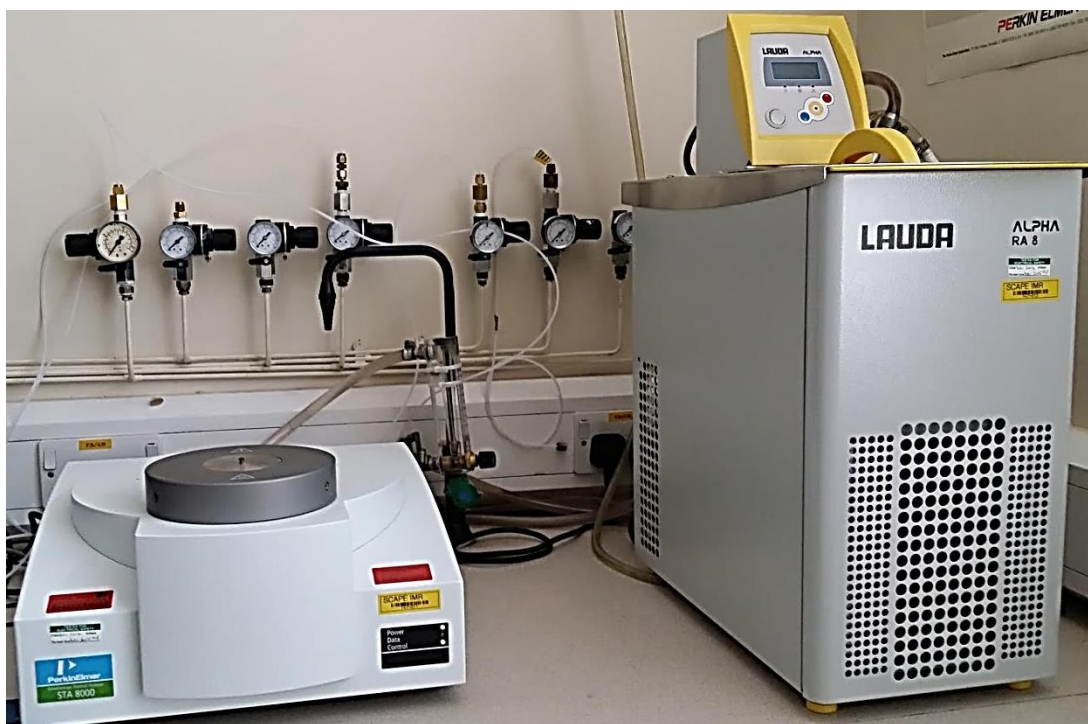
Figure 3.19: The Perkin Elmer STA 8000 and LAUDA Alpha RA 8 Chiller unit.
