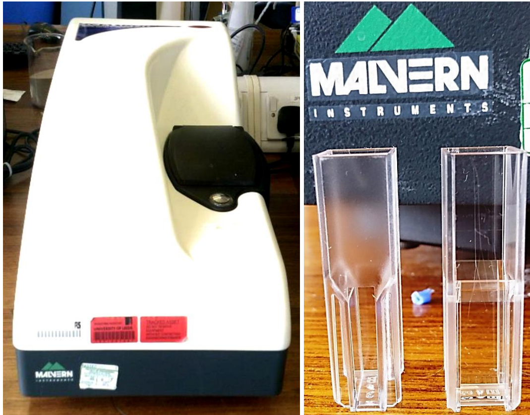
Figure 3.18: The Malvern Instruments Zetasizer Nanoseries equipment and sample cells for Dynamic Light Scattering particle size measurements.
