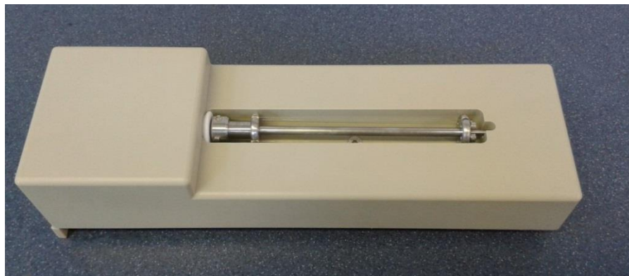
Figure 3.4: Free surface electrospinning bath with wire cylindrical electrode.
