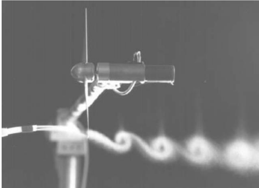
Figure 2.7 Flow visualisation experiment at TU Delft, showing tip vortices, from [25].
