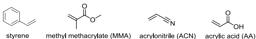
Figure 3. 10. Structures of styrene, methyl methacrylate, acrylonitrile and acrylic acid.
