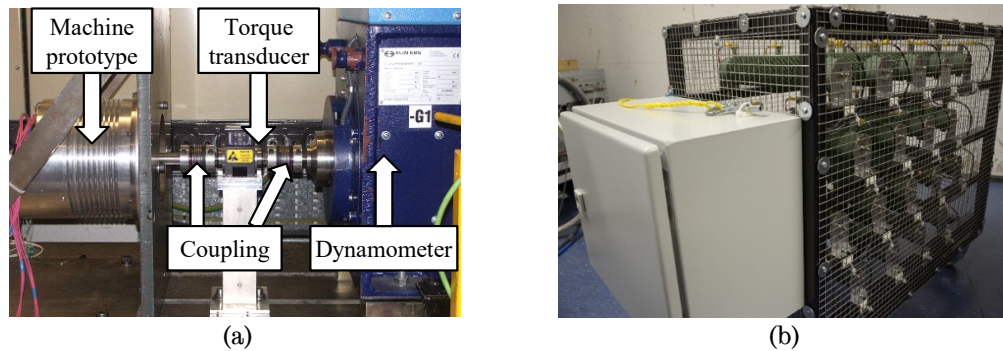
Fig. 4-35. Experimental setup. (a) Machine prototype, torque transducer, coupling and dynamometer. (b) Resistive load.
