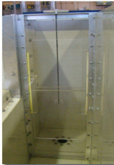
Figure 3.4 – Sluice gate that was used on both the smaller tanks to enable control of the hydraulic depth on the testing platform.
