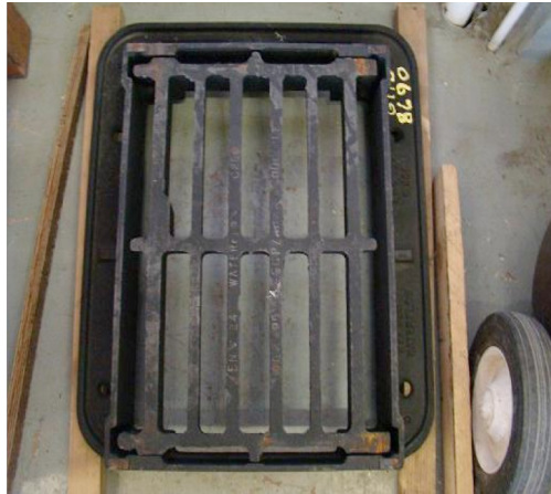
Figure 3.19 – Grate with 325mm x 437mm clear opening (HA 102 reference – S)
