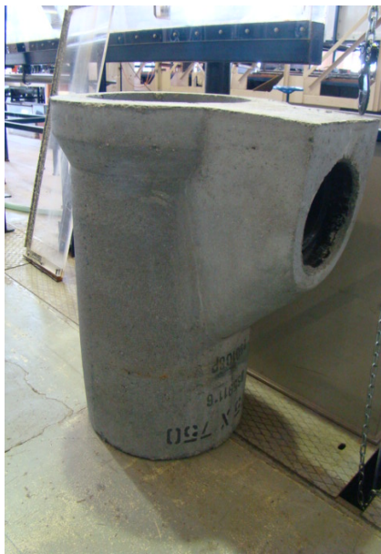
Figure 3.15 - Trapped gully with 150mm diameter outlet
