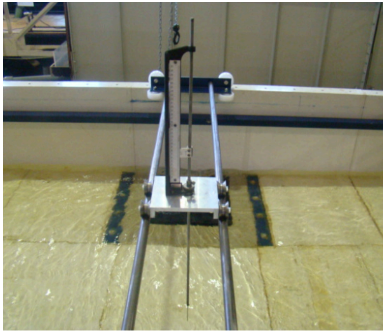
Figure 3.22 – Point-gauge measuring equipment
