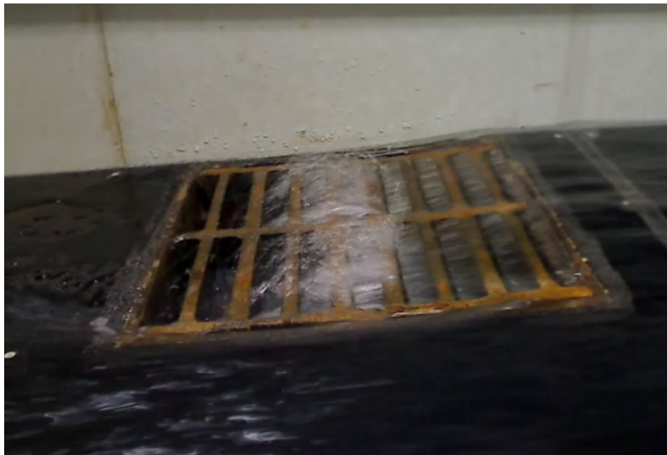
Figure 3.7 – Sloping testing platform (1/30) – detailed view of the flow onto the gully grates
