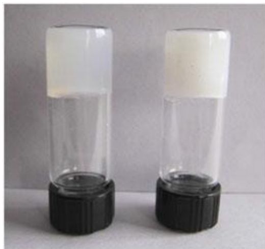
Figure 4.3.4 (a) Chemical structures of ligand 4.6 and (b) metallo-hydrogels of 4.6b / \text{Pb}^{2+}
