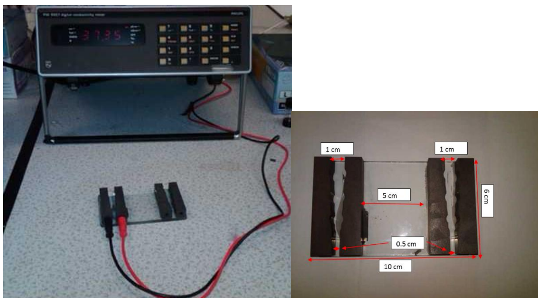
Figure 7.5.1 Fabricated in-house device for measuring the conductivity of hydrogels.
