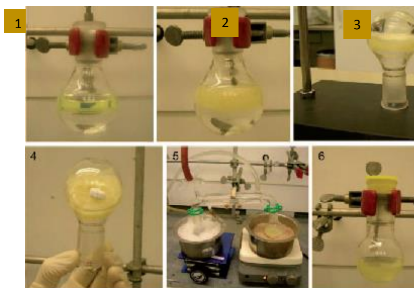
Figure 1.5.1 Gelation of bulk diesel in the presence of water, and its quantitative recovery through vacuum distillation. Photographs: 1) diesel and water form a two-phase system; 2) gel forms instantaneously upon addition of gelator by syringe; 3) Owing to the strength of the diesel gel, the flow of water is stopped upon inversion of flask; 4) Diesel gel remains after removal of the bottom water layer; 5) The entrapped diesel is recovered by vacuum distillation; 6) Recovered diesel. [Reproduced from ref. 80].
