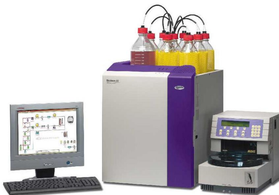
Figure 3.17: The Biochrom 30 Amino Acid Analyser (AAA) physiological system consists of a Biochrom 30 instrument (in the middle), where the analytical column is present, the Autosampler Unit (right) and a PC with the BioSys and Ezchrom Elite softwares installed.
