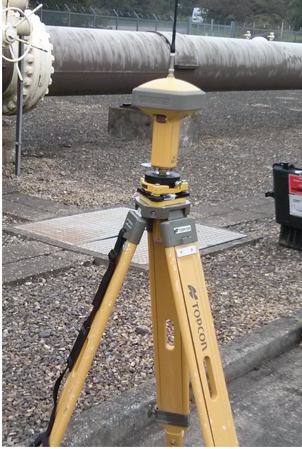
(a) Base station setup.
