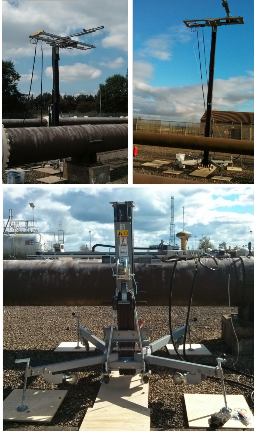
Figure 3.6: The mobile CNC measurement system deployed at the Pannal site.
