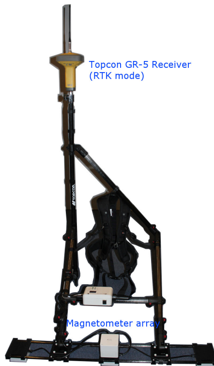
Figure 6.2: The assembled UNISCAN instrument.
