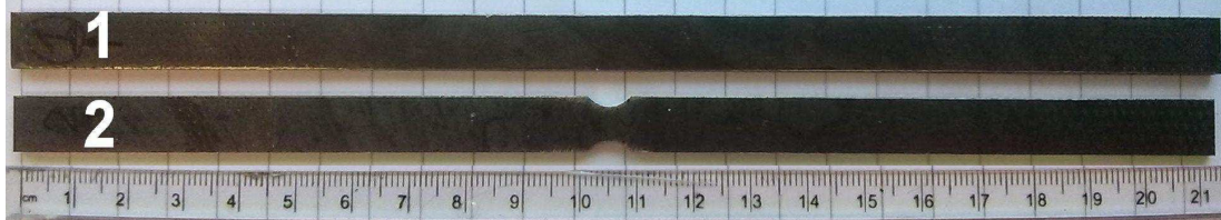
Figure 3.10: Steel samples used in the experiment. The stressed section was from 45 mm to 165 mm.
