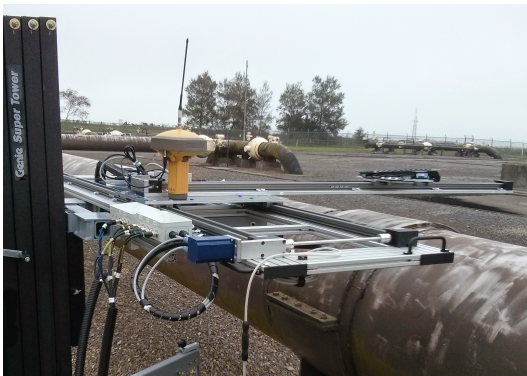
(a) Use of the rover on the Y arm to position the measurement plane.
