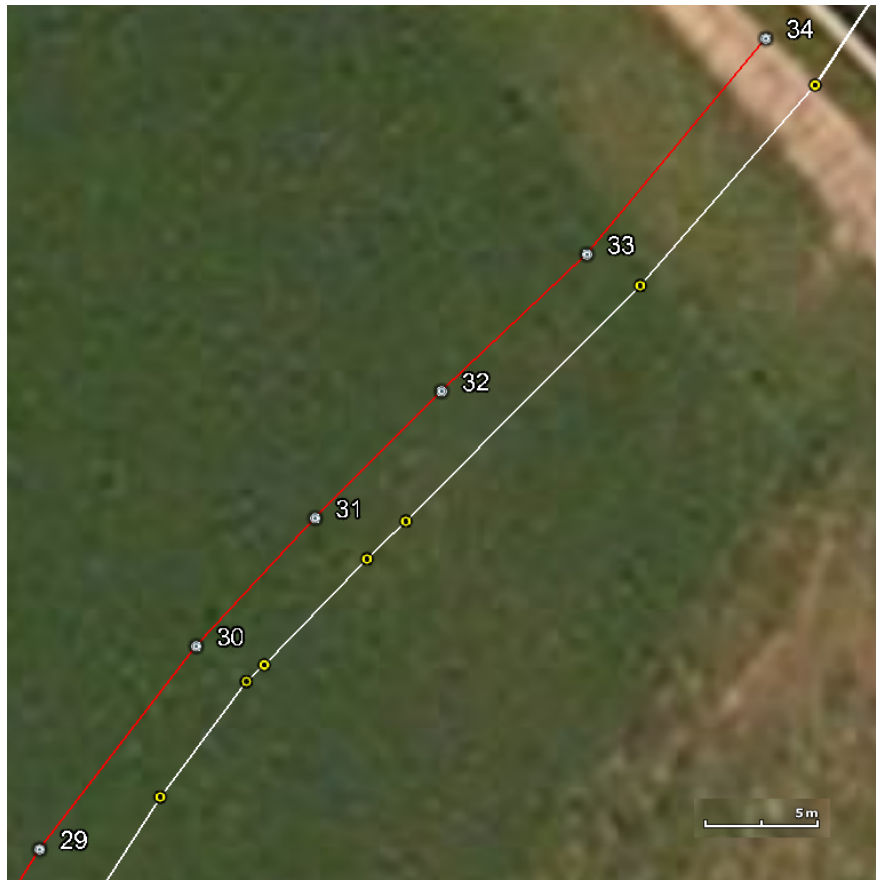
Figure 6.4: A comparison between the ILI and the SCT mapping data of the PANE29 pipeline. White : the ILI mapping data; Red : the SCT mapping data. Because of different positioning methods the conversions between OSGB36 and WGS84, the distance between two lines was approximately 3 m.
