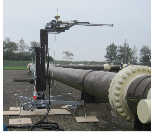
(b) Use of the mobile CNC-based measurement system on the 30-inch pipeline.
