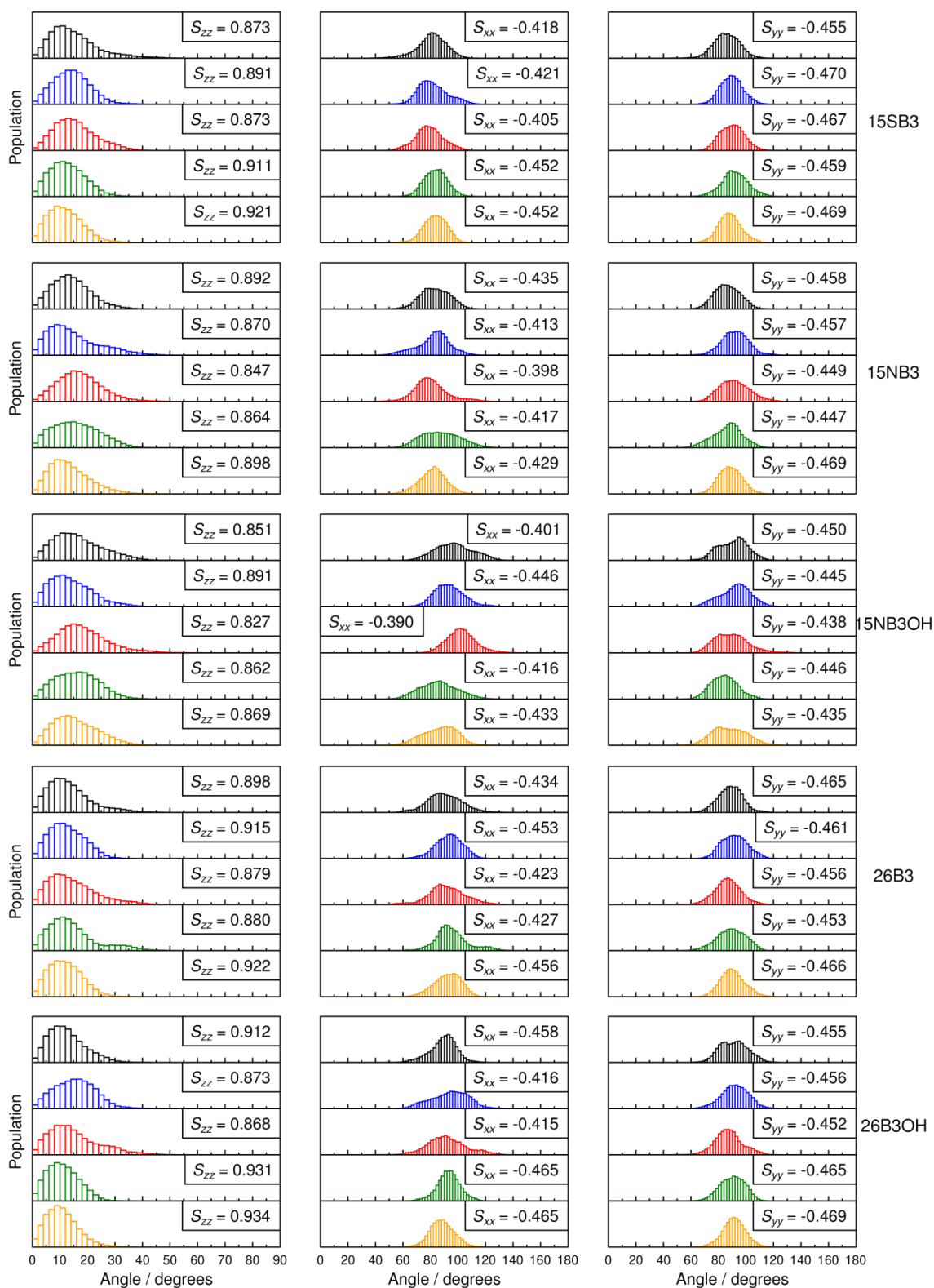
Figure 5.12 Histograms of the angles made between the principal, secondary and tertiary surface axes and the host director, of individual dye molecules (represented by different colours, consistent with those used in Chapter 4) measured from the five guest-host simulations.
