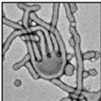
Figure 1.16: A TEM micrograph showing a “Jellyfish” structure, composed of the copolymer Poly([2-methacryloyl-oxy]ethyl phosphorylcholine)-block-poly(2-[diisopropyl- amino]ethyl methacrylate) (PMPC-PDPA). These structures are rarely trapped by the process routes used in this thesis, however other formation processes such as polymerisation-induced self-assembly allow for the study of such structures in greater detail. Scale bar = 200 nm.
