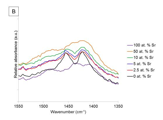
Figure 5.16. FTIR-ATR spectra of unsintered strontium-substituted nHA powders (0, 2.5, 5, 10, 50 and 100 at. % Sr) produced using optimised method 1. (A) 1150 – 900 cm<sup>-1</sup>: phosphate group bands. (B) 1550 - 1350 cm<sup>-1</sup>: carbonate group bands.
