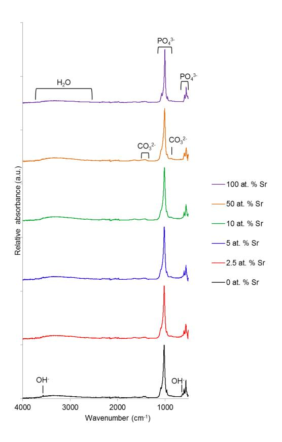
Figure 5.15. FTIR-ATR spectra of unsintered strontium-substituted nHA powders (0, 2.5, 5, 10, 50 and 100 at. % Sr) produced using optimised method 1.
