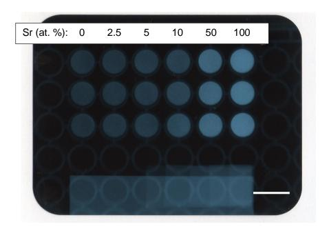
Figure 5.19. Radiograph of strontium-substituted nHA powders (0, 2.5, 5, 10, 50 and 100 at. % Sr) produced using optimised method 1, n=3, with aluminium step wedge used for quantification. Scale bar = 1 cm.
