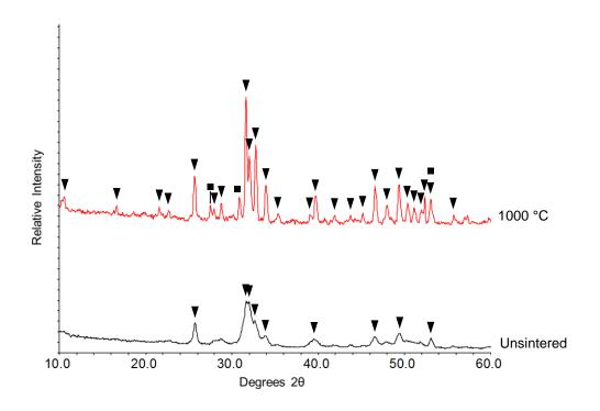
Figure 5.5. XRD patterns of nHA powder prepared using method 3. The unsintered sample (black) and sample sintered at 1000 °C for 2 h (red) are displayed. Peak labels: ▼ hydroxyapatite; ■ β-tricalcium phosphate.
