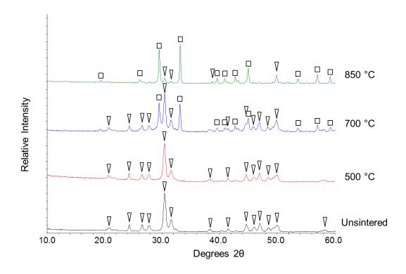
Figure 5.22. XRD patterns of 100 at. % strontium-substituted nHA powder produced using optimised method 3: unsintered and sintered at 500, 700 and 850 °C. Peak labels:  $^{\sqrt{}}$  strontium hydroxyapatite;  $\Box$   $\beta$ -tristrontium phosphate.
