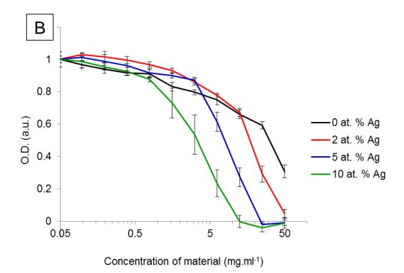
Figure 5.50. Optical density of *S. aureus* (A) and *P. aeruginosa* (B) in suspension culture at 20 h incubated with 0, 2, 5 and 10 at. % silver-doped nHA paste (paste material control subtracted) (n = 9). Error bars  $\pm$  standard error of the mean.
