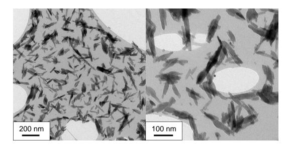
Figure 5.2. TEM micrographs of unsintered nHA powder prepared by method 1.
