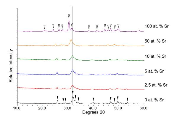
Figure 5.12. XRD patterns of unsintered strontium-substituted HA powders (0, 2.5, 5, 10, 50 and 100 at. % Sr) produced using optimised method 1. Peak labels: Number of the produced using optimised method 1. Peak labels: Number of the produced using optimised method 1. Peak labels:
