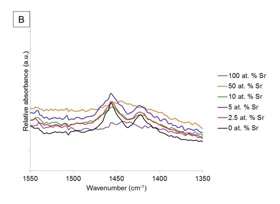
Figure 5.25. FTIR-ATR spectra of unsintered strontium-substituted nHA powders (0, 2.5, 5, 10, 50 and 100 at. % Sr) produced using optimised method 3. (A) 1150 – 900 cm<sup>-1</sup>: phosphate group bands. (B) 1550 - 1350 cm<sup>-1</sup>: carbonate group bands.
