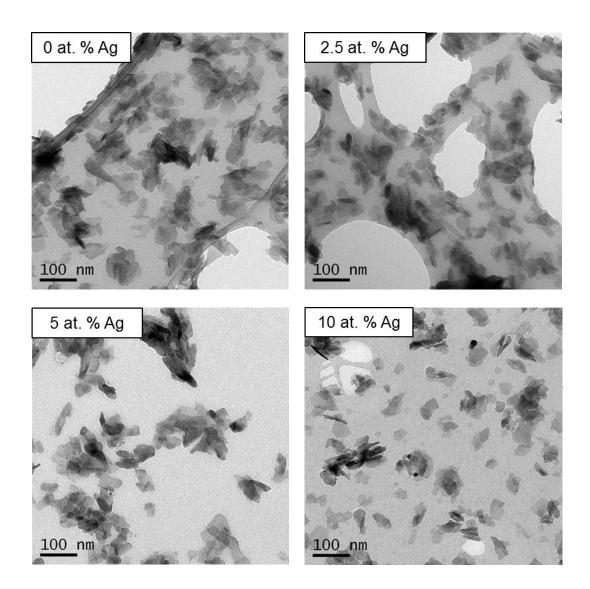
Figure 5.30. TEM micrographs of unsintered silver-doped nHA powders (0, 2, 5 and 10 at. % Ag) produced using altered method 1.
