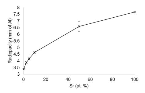
Figure 5.27. Quantification of radiopacity of strontium-substituted nHA powders (0, 2.5, 5, 10, 50 and 100 at. % Sr) produced using optimised method 3, n=3. Error bars:  $\pm$  S.D.
