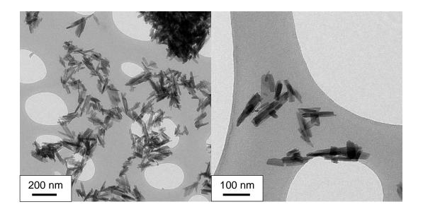
Figure 5.4. TEM micrographs of unsintered nHA powder prepared using method 2.
