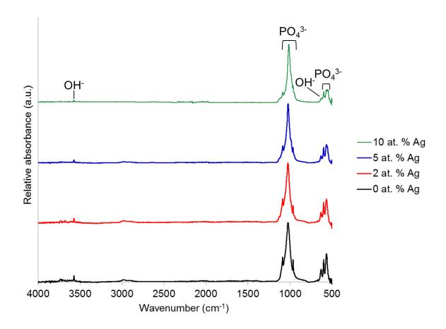
Figure 5.33. FTIR-ATR spectra of silver-doped nHA powders (0, 2, 5 and 10 at. % Ag) sintered at 1000 °C for 2 h produced using altered method 1.
