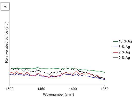
Figure 5.34. FTIR-ATR spectra of silver-doped nHA powders (0, 2, 5 and 10 at. % Ag) sintered at 1000 °C for 2 h produced using altered method 1. (A) 1150 – 900 cm<sup>-1</sup>: phosphate group bands. (B) 1550 - 1350 cm<sup>-1</sup>: carbonate group bands.
