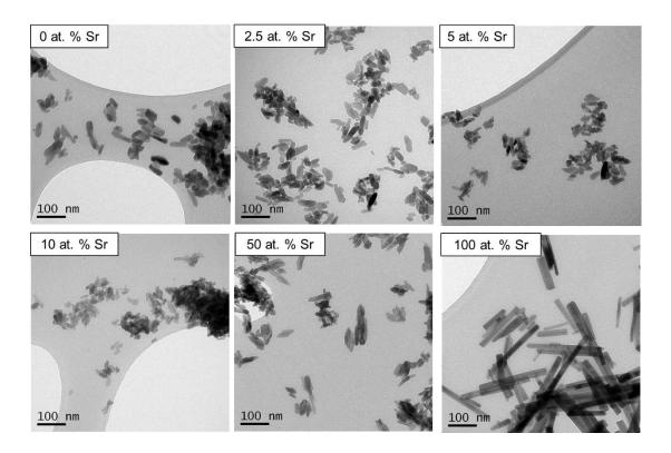
Figure 5.23. TEM micrographs of unsintered strontium-substituted HA powders (0, 2.5, 5, 10, 50 and 100 at. % Sr) produced using optimised method 3.
