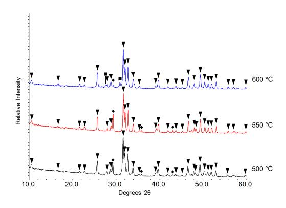
Figure 5.8. XRD patterns of nHA powder prepared using method 4 at pH 10. The samples sintered at 500 (black), 550 (red) and 600°C for 2 h (blue) are displayed. Peak labels: ▼ hydroxyapatite; ■ β-tricalcium phosphate; ◆ ammonium nitrate.
