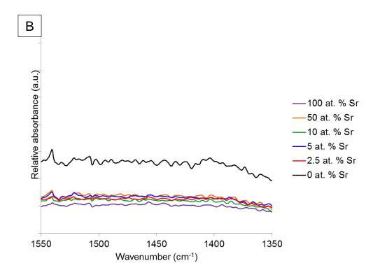
Figure 5.18. FTIR-ATR spectra of strontium-substituted nHA powders (0, 2.5, 5, 10, 50 and 100 at. % Sr) sintered at 1000 °C for 2 h produced using optimised method 1.
