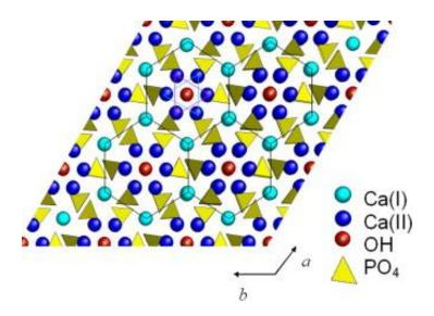
Figure 2.2. Hydroxyapatite crystal structure viewed along the c-axis. Note the different positions of Ca(I) and Ca(II). Reproduced with permission from reference [9].
