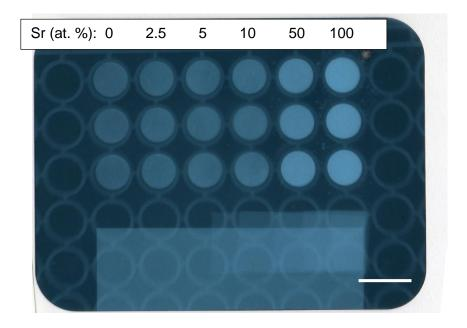
Figure 5.26. Radiograph of strontium-substituted nHA powders (0, 2.5, 5, 10, 50 and 100 at. % Sr) produced using optimised method 3, n=3, with aluminium step wedge used for quantification. Scale bar = 1 cm.
