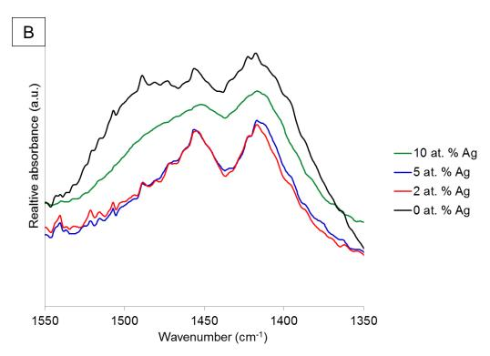
Figure 5.32. FTIR-ATR spectra of unsintered silver-doped nHA powders (0, 2, 5 and 10 at. % Ag) produced using altered method 1. (A) 1150 – 900 cm<sup>-1</sup>: phosphate group bands. (B) 1550 - 1350 cm<sup>-1</sup>: carbonate group bands.
