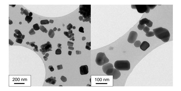
Figure 5.9. TEM micrographs of nHA powder sintered at 550 °C prepared using method 4 at pH 10.
