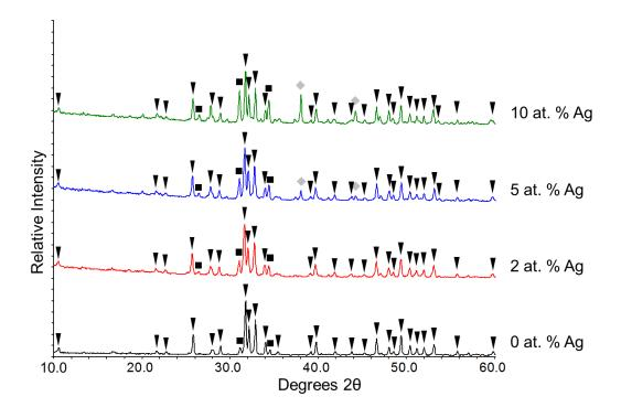
Figure 5.29. XRD patterns of silver-doped nHA powders (0, 2, 5 and 10 at. % Ag) produced using altered method 1 sintered at 1000 °C for 2 h. Peak labels:
