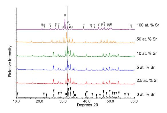
Figure 5.13. XRD patterns of strontium-substituted HA powders (0, 2.5, 5, 10, 50 and 100 at. % Sr) produced using optimised method 1 sintered at 1000 °C for 2 h. Peak labels:  $\P$  hydroxyapatite;  $\blacksquare$   $\beta$ -tricalcium phosphate;  $\P$  strontium hydroxyapatite;  $\square$   $\beta$ -tristrontium phosphate.
