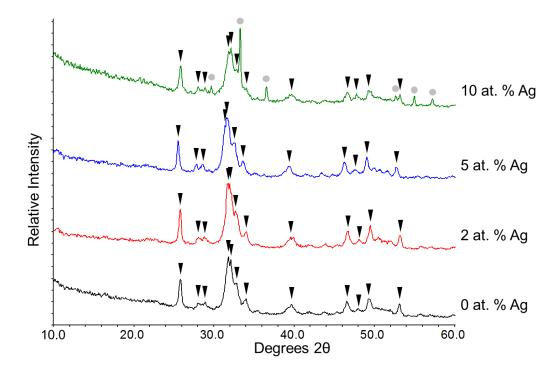
Figure 5.28. XRD patterns of unsintered silver-doped nHA powders (0, 2, 5 and 10 at. % Ag) produced using altered method 1. Peak labels: hydroxyapatite; silver phosphate.
