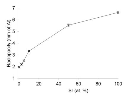
Figure 5.20. Quantification of radiopacity of strontium-substituted nHA powders (0, 2.5, 5, 10, 50 and 100 at. % Sr) produced using optimised method 1, n=3. Error bars:  $\pm$  S.D.
