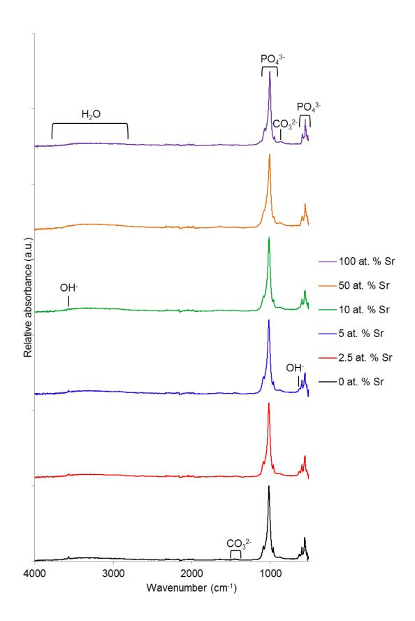
Figure 5.24. FTIR-ATR spectra of unsintered strontium-substituted nHA powders (0, 2.5, 5, 10, 50 and 100 at. % Sr) produced using optimised method 3.
