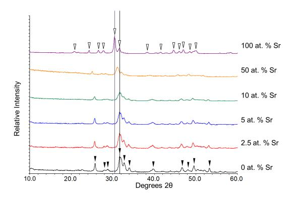
Figure 5.21. XRD patterns of unsintered strontium-substituted nHA powders (0, 2.5, 5, 10, 50 and 100 at. % Sr) produced using optimised method 3. Peak labels: hydroxyapatite;
