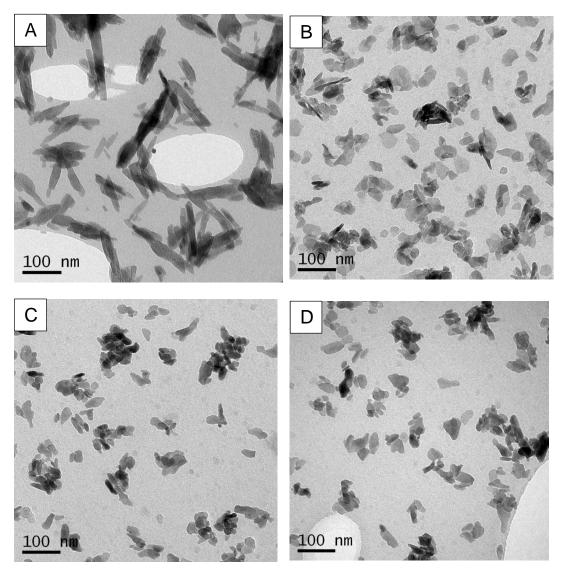
Figure 5.10. TEM micrographs showing particle morphology when incremental changes were made using method 1: (A) original method (1-A); (B) Phosphoric acid solution addition rate increased (1-B); (C) Reaction performed at room temperature (1-C); (D) Increased concentration of reaction (1-D).
