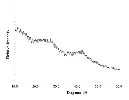
Figure 5.7. XRD pattern of unsintered powder prepared using method 4 at pH 10. No identifiable crystalline phases were detected.
