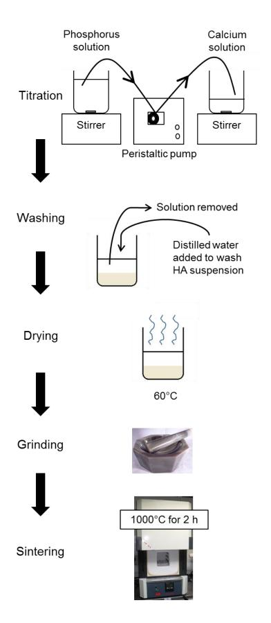
Figure 4.1. Schematic diagram showing production stages for method 1-3.
