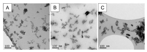
Figure 5.11. TEM micrographs displaying particle morphology when incremental changes were made using method 3: (A) Original method (3-A); (B) Phosphorus solution addition rate increased (3-E); (C) Increased concentration of reactants (3-F).
