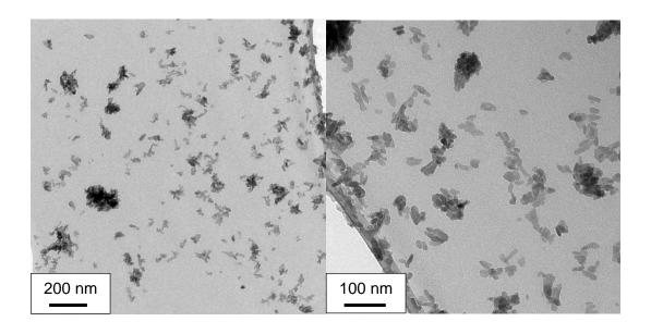
Figure 5.6. TEM micrographs of unsintered nHA powder prepared using method 3.
