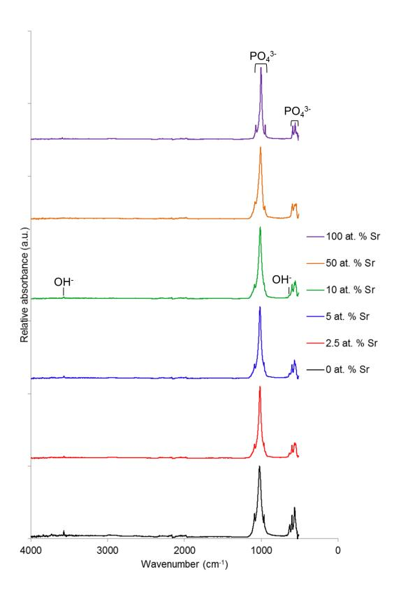
Figure 5.17. FTIR-ATR spectra of strontium-substituted nHA powders (0, 2.5, 5, 10, 50 and 100 at. % Sr) sintered at 1000 °C for 2 h produced using optimised method 1.
