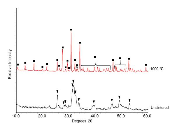
Figure 5.3. XRD patterns of nHA powder prepared using method 2. The unsintered sample (black) and sample sintered at 1000 °C for 2 h (red) are displayed. Peak labels: ▼ hydroxyapatite; ■ β-tricalcium phosphate.
