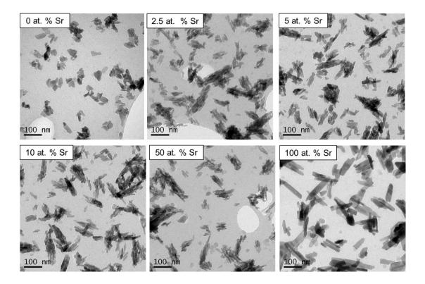
Figure 5.14. TEM micrographs of unsintered strontium-substituted HA powders (0, 2.5, 5, 10, 50 and 100 at. % Sr) produced using optimised method 1.
