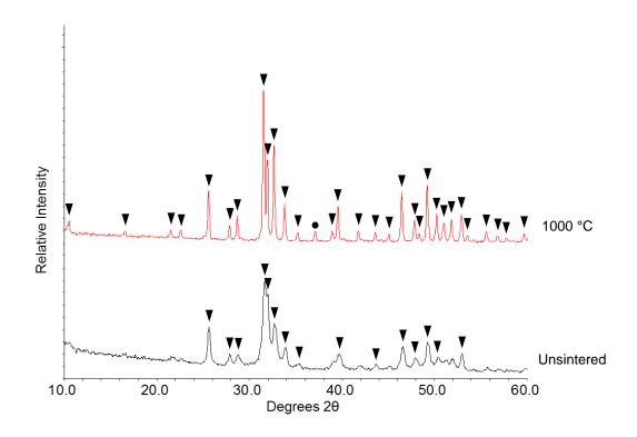
Figure 5.1. XRD patterns of nHA powder prepared by method 1. The unsintered sample (black) and sample sintered at 1000 °C for 2 h (red) are displayed. Peak labels: ▼ hydroxyapatite; ● calcium oxide.
