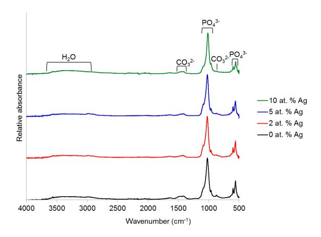
Figure 5.31. FTIR-ATR spectra of unsintered silver-doped nHA powders (0, 2, 5 and 10 at. % Ag) produced using altered method 1.
