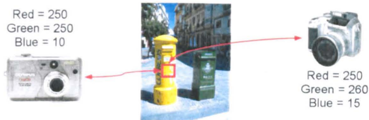
Figure 2-36: An example of device-dependent values. Different cameras give different RGB values from the same scene.
