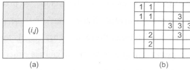
Figure 5-23: (a) The position of 8-neighboring pixels of a pixel at coordinates (i, j) (8 shadowed cells). (b) An Example of a labelled image. It indicates three connected components in an image.
