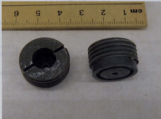
Figure 3.9 Photograph of anode plug
