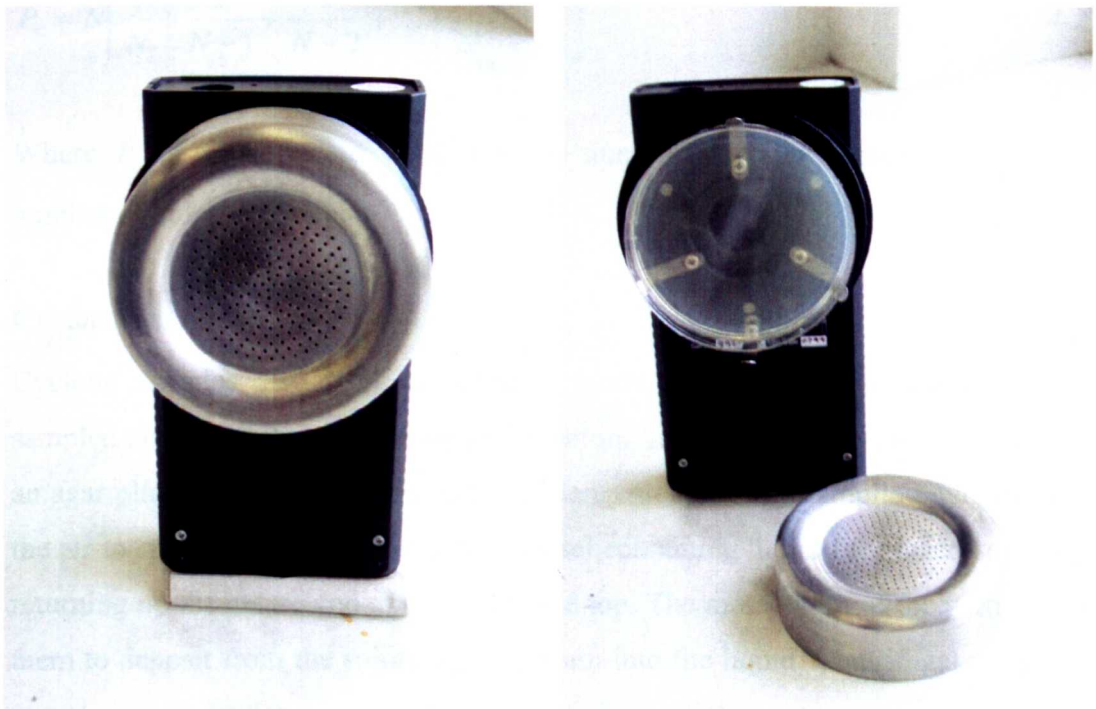
Figure 4-4: Photograph of MicroBio MB2 Air Sampler, showing the sieve head (left) and the positioning of the Agar plate (right)
