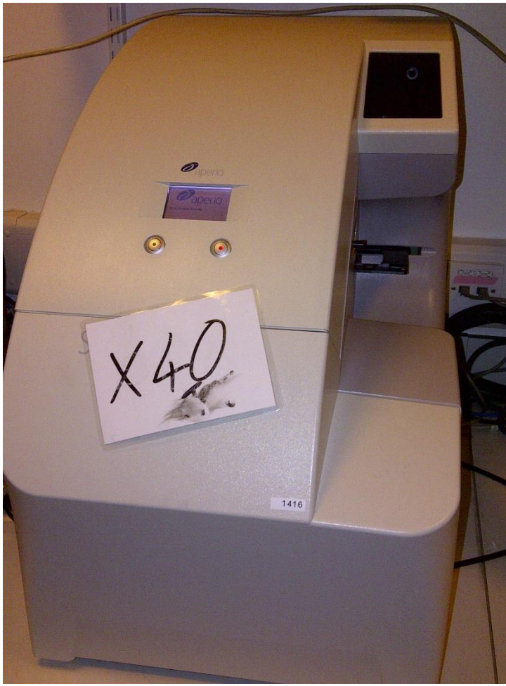
Figure 2.68 : Slides were digitised using an Aperio Scanscope and the images stored on a server for quantitative histological analysis using 20x magnification sections analysed using Aperio Imagescope v.10.2.2.2319 (Aperio technologies, Inc. Vista, CA, USA)
