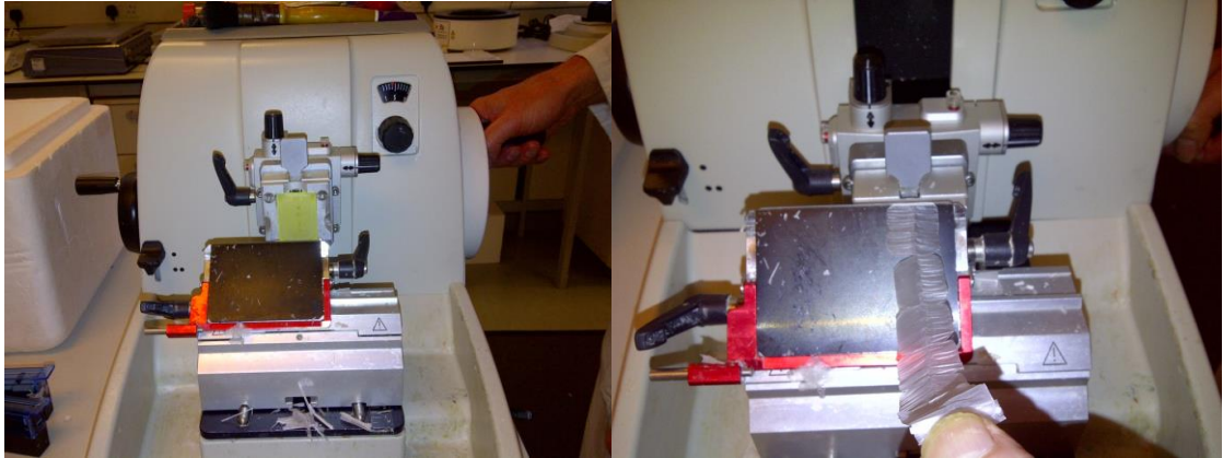
Figure 2.65: Tissue was sectioned transversely at 4 \mu m using a Leica RM 2235 microtome
