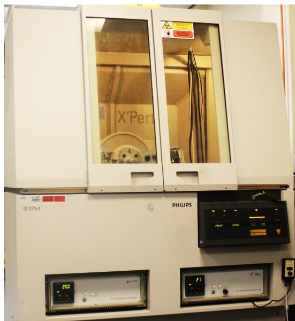
Figure 5-9 PHILIPS X'PERT 1 X-ray diffractometer used for XRD analysis
