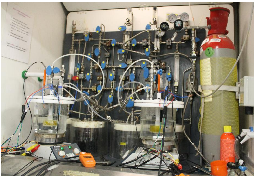
Figure 5-6 A picture of the sour corrosion test set up while in use.
