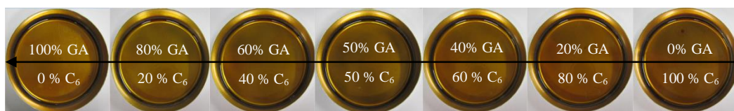
Figure 3.13 Samples of ELO cured with different compositions of glutaric anhydride and adipic acid. (Originally in colour)
