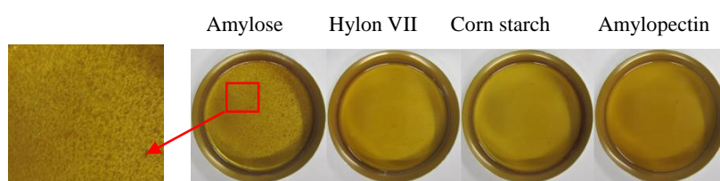
Figure 4.6 Samples containing 10 wt% different starches cured at 140 °C for 8 h. (Originally in colour)
