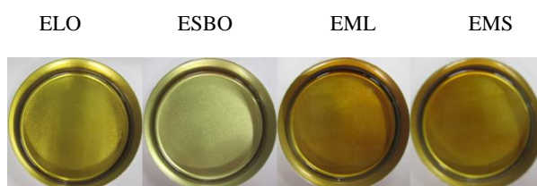
Figure 2.4 Different epoxy prepolymers cured with adipic acid at 160 °C for 1 h. (Originally in colour)
