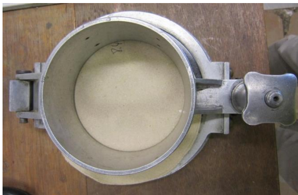
Figure 5.3 Water adsorption capacity test for cardboards
