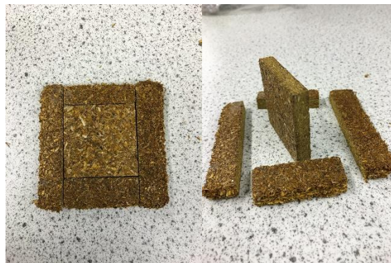
Figure 3.3 Final bioboards cutting for 5 cm X 5cm pieces
