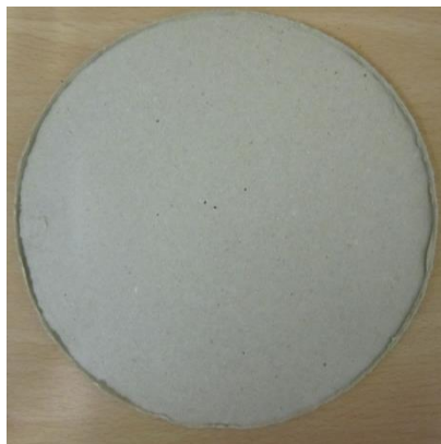
Figure 4.1 Lab-scale cardboard with pulp and wheat straw powder
