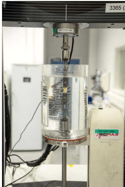
Fig 2.6 – Instron 3365 test rig with Instron Biobath set at 37 °C with tissue clamped in custom made grips undergoing the test procedure.
