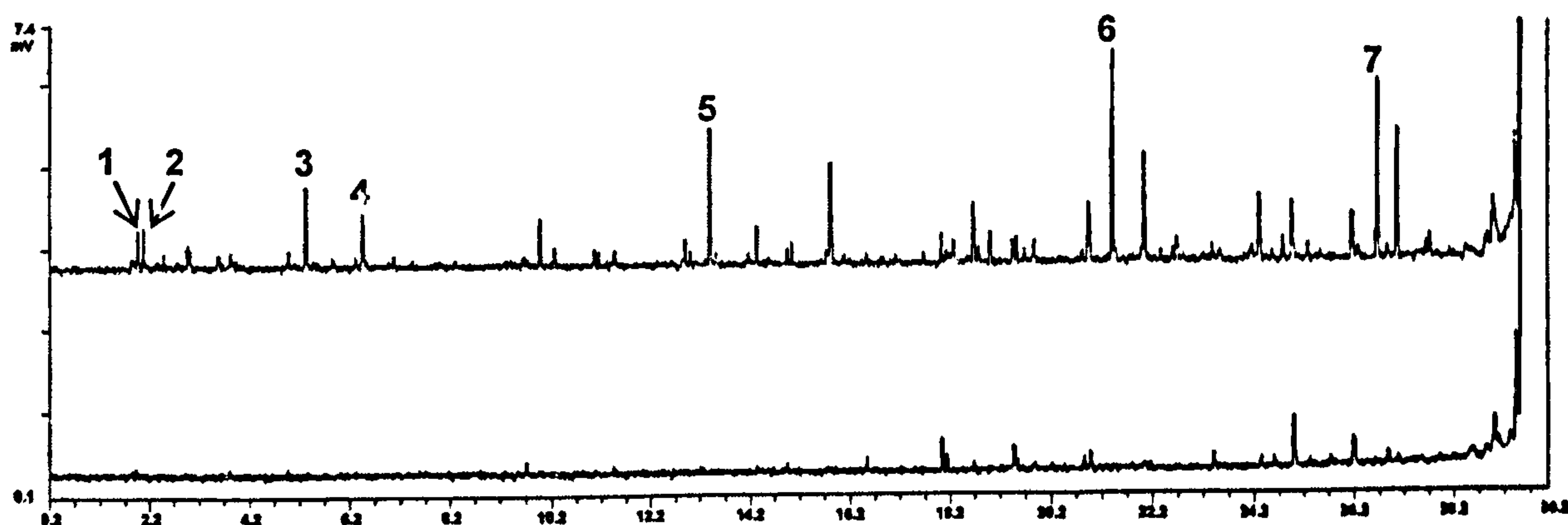
Figure B.8: GC traces of unoxidised (bottom trace) and oxidised (top trace) squalane at 200 °C for 9 minutes in static intermediate reactor – part 1 (0 to 30 minutes). Peaks 1: propanone; 2: 2-methylpentane; 3: 6-methyl-2-heptanone; 4: 2,6-dimethylnonane; 5: 6,10-dimethyl-2-undecanone; 6: 7,11,15-trimethyl-2-hexadecanone; and 7: 6,11,15,19-tetramethyl-2-eicosanone
