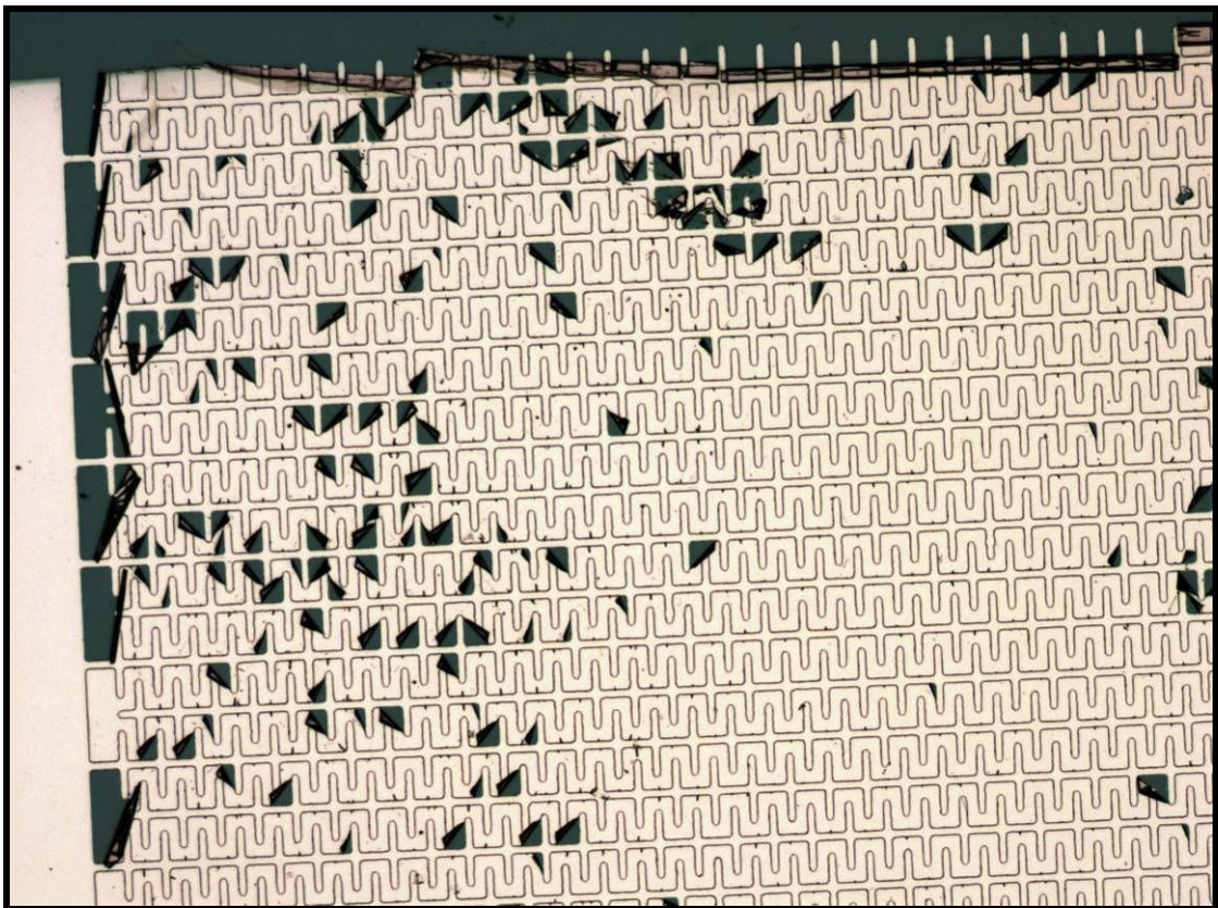
Fig. 139. Sample 1 – Design 5 (Example of poor lift off)
