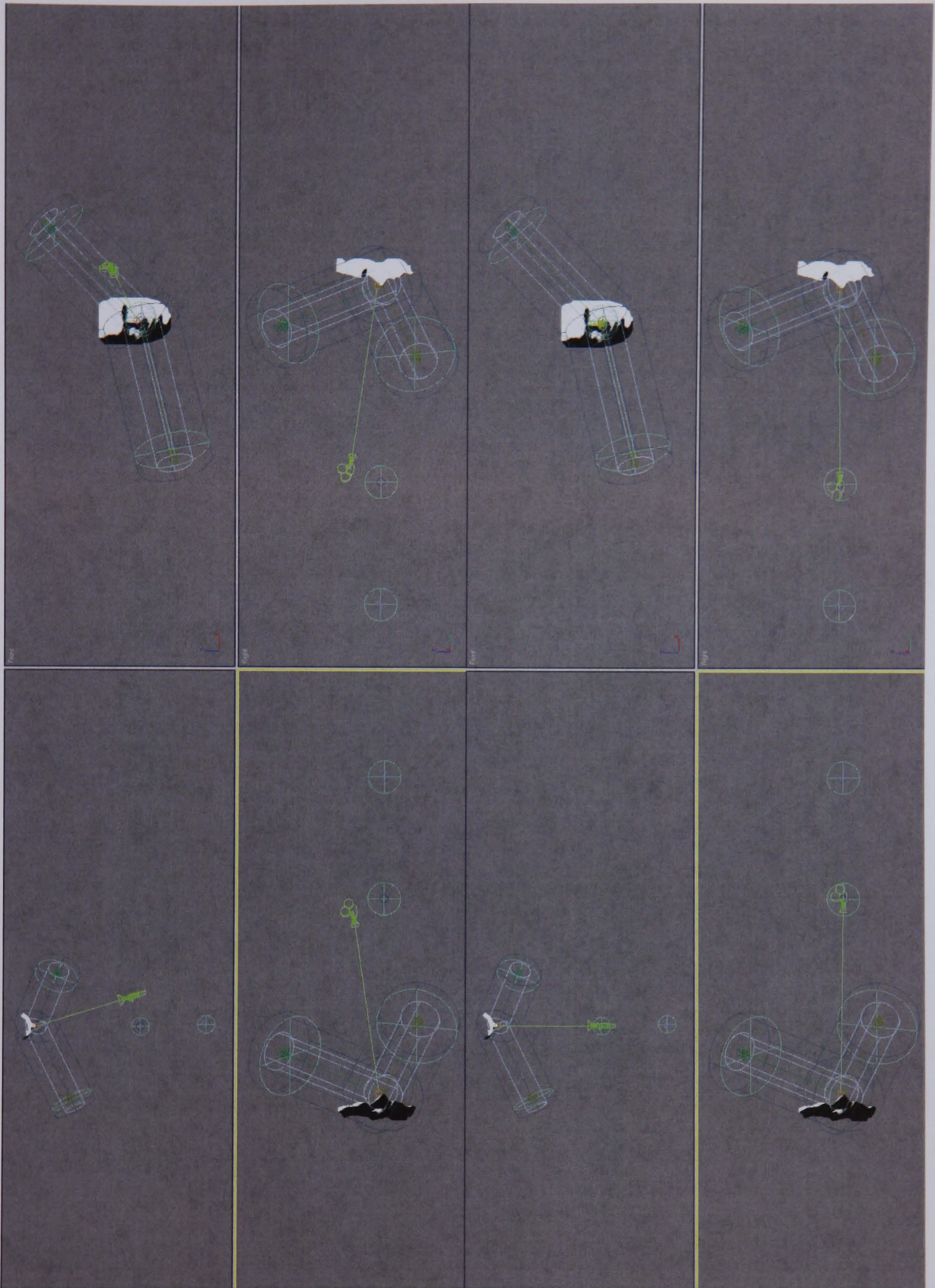
Figure 1.4: The render set-up used to generate the images. The cylinders represent directional lighting. Lights were enabled and disabled in order to generate the illumination conditions, and the camera moved between the positions shown to generate the pose conditions
