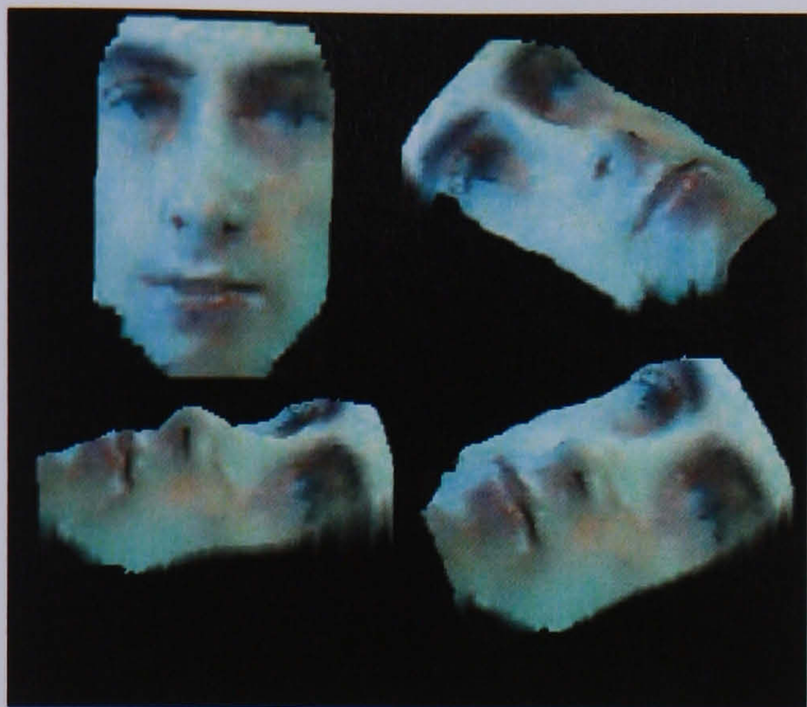
Figure 11. Four views of a face coded in a total of less than 1kbyte.
