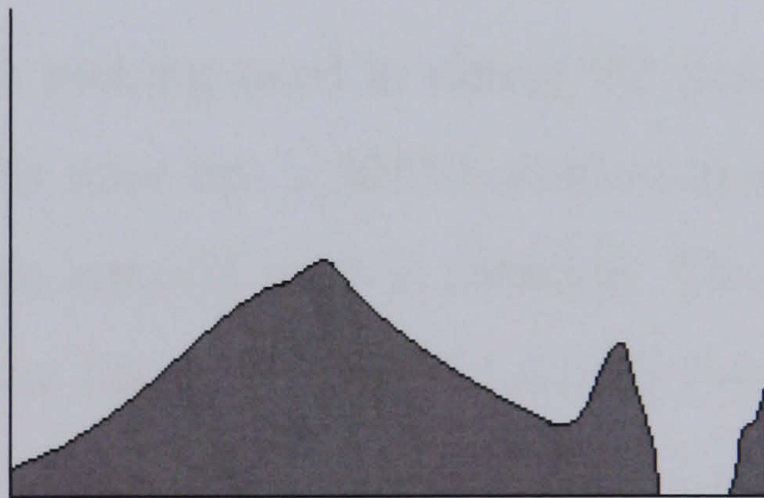
Figure 3.10: Sketch of an image histogram with an isolated peak. This peak is highly unlikely to contain useful face data, and can be quantised out, removing the wasted quantisation levels falling in the gap between it and the body of the data in the image
