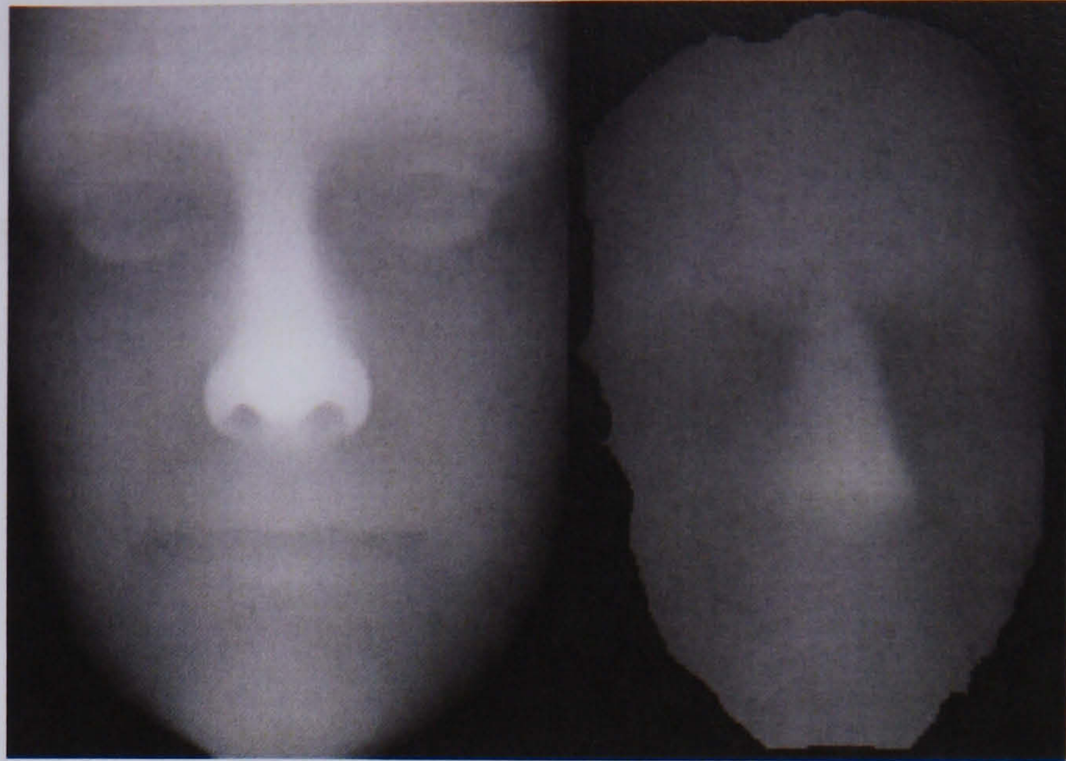
Figure 3.7: Notre Dame depth maps (left) captured with a laser scanner are of a much higher quality than the York depth maps (right) captured with a patterned light projector with shape-from-stereo
