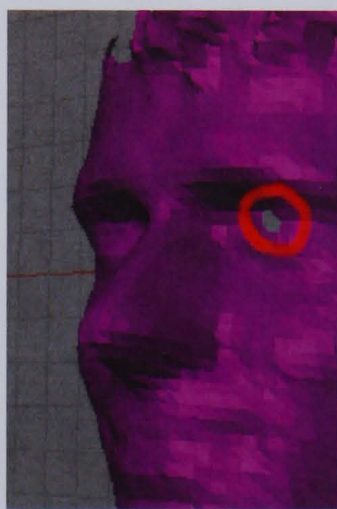
Figure 3.4: A point of error caused by specular reflection in the mesh in the eye Figure 3.5: Gaps in the mesh Figure 3.6: Disconnected sections of model "free floating" from the face
