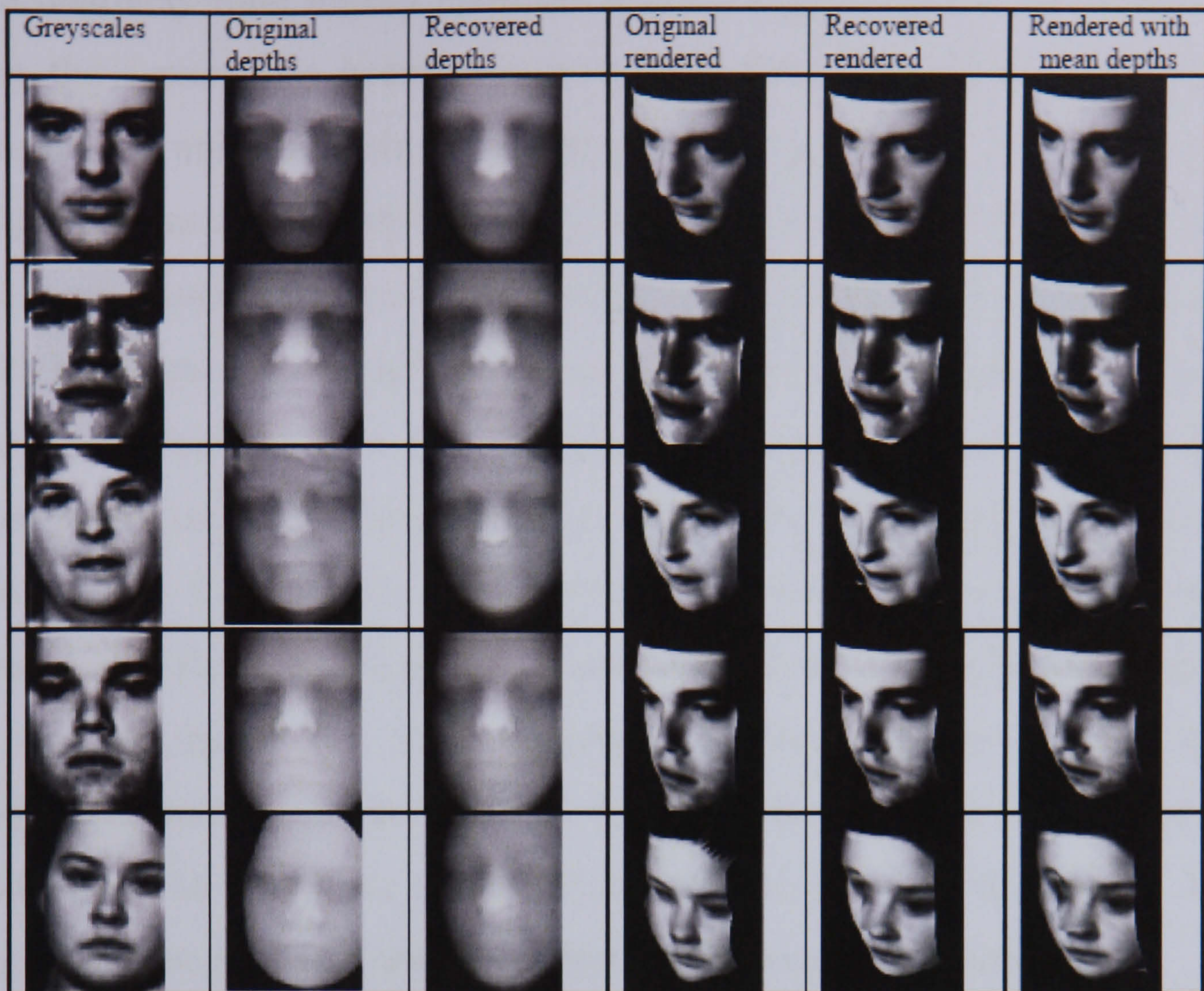
Figure 4.1: Examples of the output of the estimator. The left hand images are the original textures used as probes, the next images are the ground-truth depth maps for these images, as captured by a laser scanner. The next images are the estimated depth maps. Finally, a render with the original model, a “reconstruction” of this scene using the estimated model and the same reconstruction using the global mean face are presented for comparison. The original texture is mapped on to the models in all cases. Of interest are the second sample, showing a marked tolerance to the luminance noise in the source image, and the fifth sample, which demonstrates poor performance on a badly oriented and centred image.
