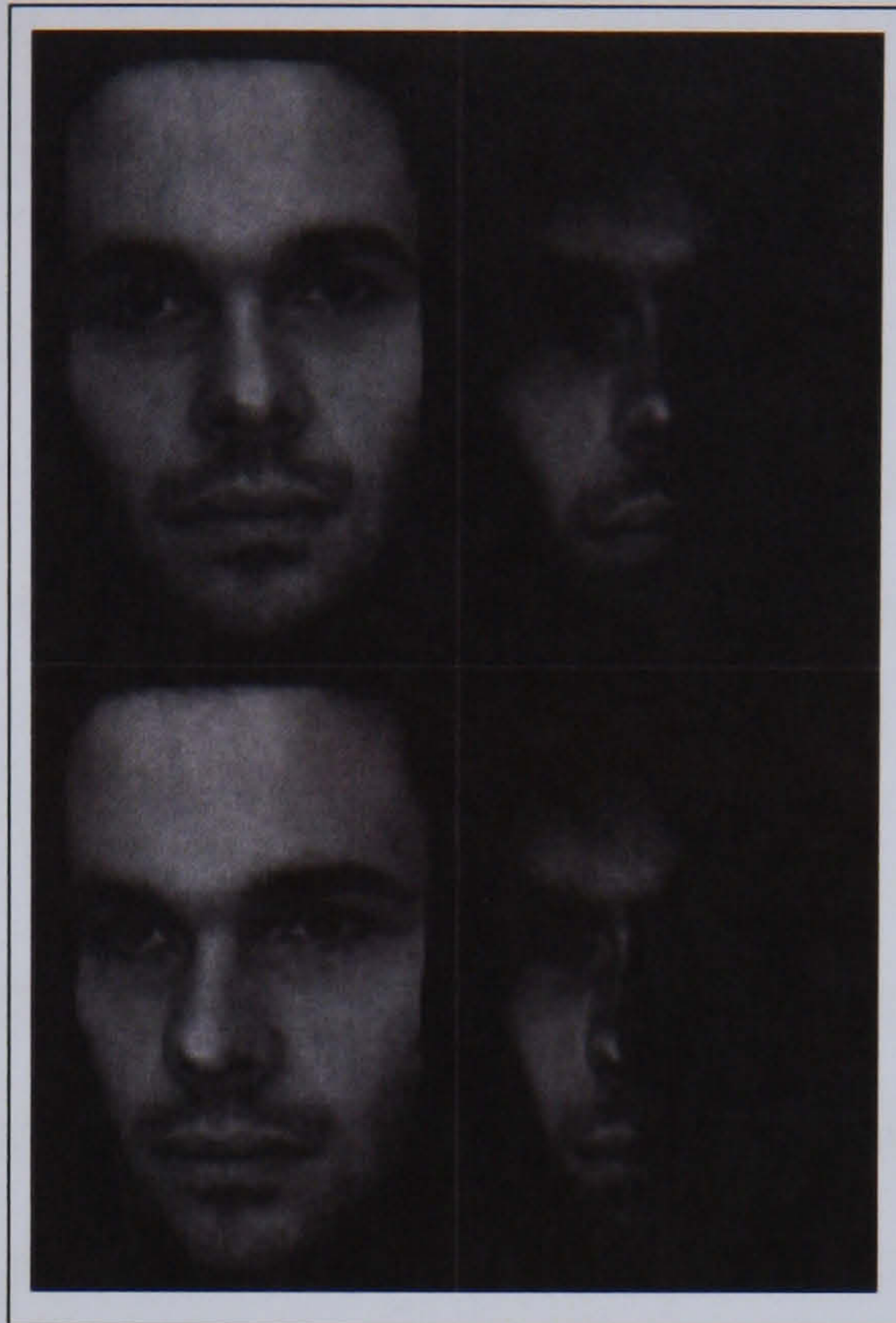
Figure 1.2: A 3d model made from a frontal view of a face, in the lower pictures the model has been rotated slightly. In the left hand, unshaded images, the lines where the model creation has failed as the face surface angles away from the camera are evident. Using strong directional illumination to shade the face, as shown in the right hand-column, minimises the perceptual effect of these edges at the cost of generating a slightly "theatrical" image.
