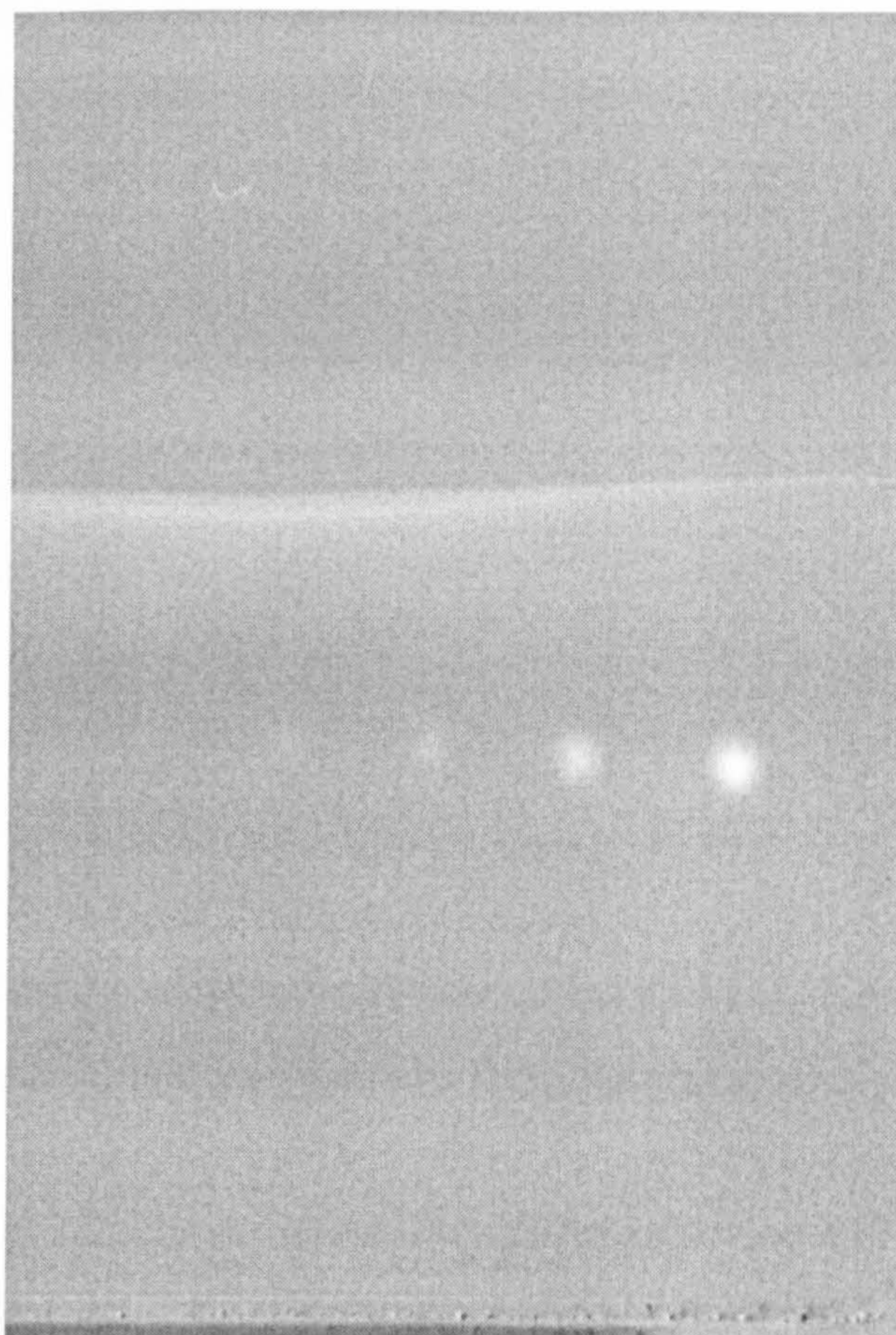
Figure 2.9 Referenced image of Sudan II at 50, 25, 10 and 5 ng on a wet plate run with DCM imaged using the blue additive filter. Only white spots are present as the background image used was of the wet blank plate, not a spotted plate. Notice that the signal referencing at the solvent front produces a white irregular band. This is due to the solvent front being in a slightly different position in both images.
