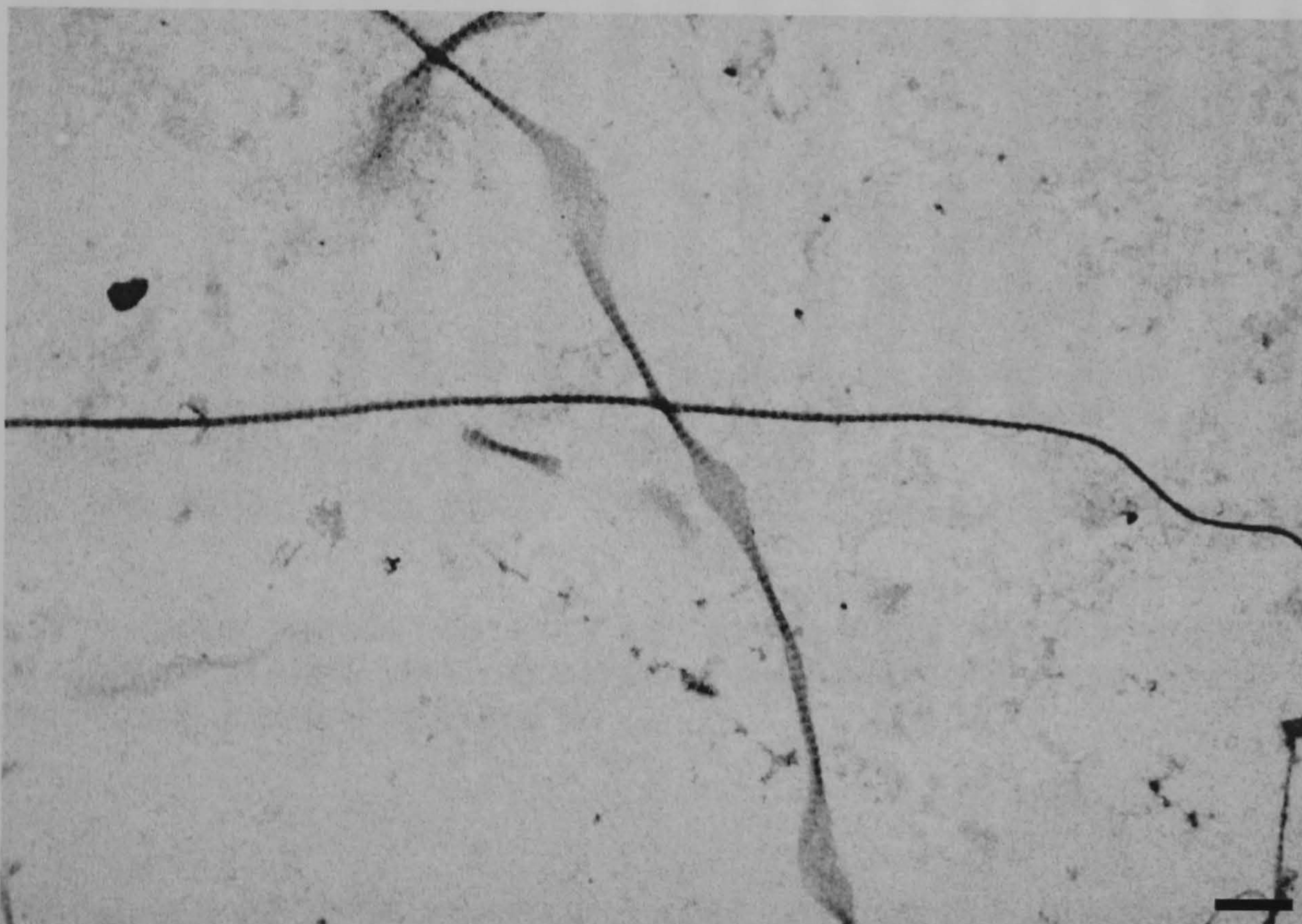
Figure 5.5 A TEM image showing a heat damaged collagen fibril with regions of Beaded alteration. The scale bar is 500 nm.
