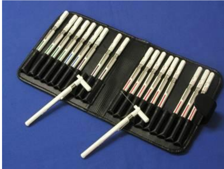
Figure 3.1 Semmes Weinstein Monofilaments (SWM) kit which consists of 20 different monofilament starting from 0.008 g force up to 300 g increasing with logarithmic increments.
