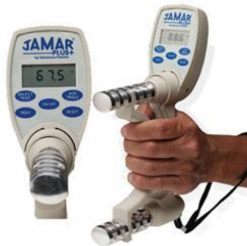
Figure 4.6 Maximum hand grip force measurement device, JAMAR handheld dynamometer with adjustable levels for the panellist/patients convenience. There is a digital screen on the dynamometer which shows the maximum force applied.
