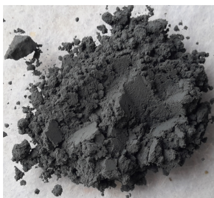
Figure 3.4 – An optical image of the \text{CuAlO}_2 powder obtained during the synthesis.
