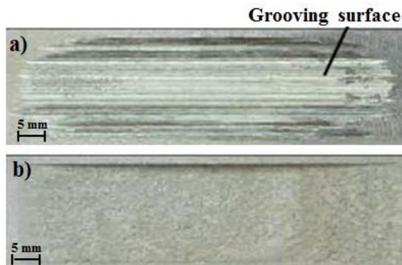
Figure 9.17. Wear mechanism observed with full test rig with abradable material AlSi-hBN and titanium blade (Ti-6Al-4V), a) Low incursion rate; b) High incursion rate (Data provided by Rolls Royce Surface Engineering Group).
