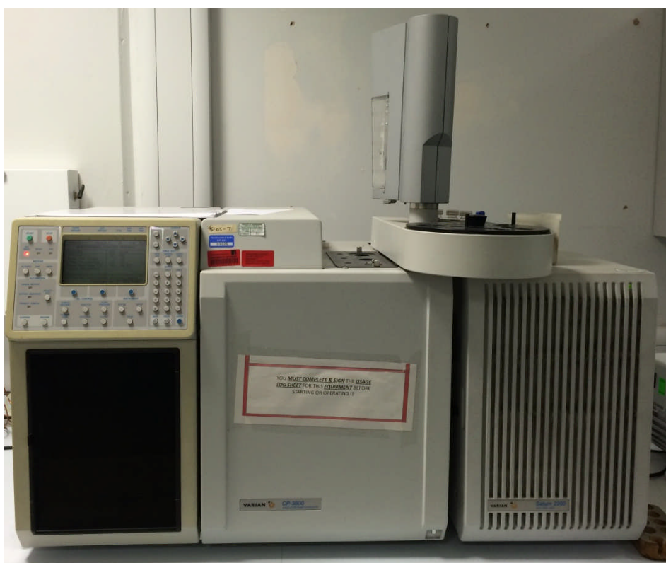
Figure 3.5.2 GC/MS analyzer used for the analyses of liquid effluent
