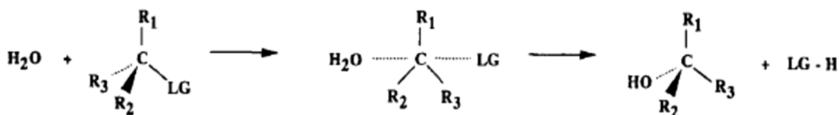
Figure 2.3.2 General reaction pathway for hydrolysis in supercritical water (LG: leaving group) adapted from ref [28]
