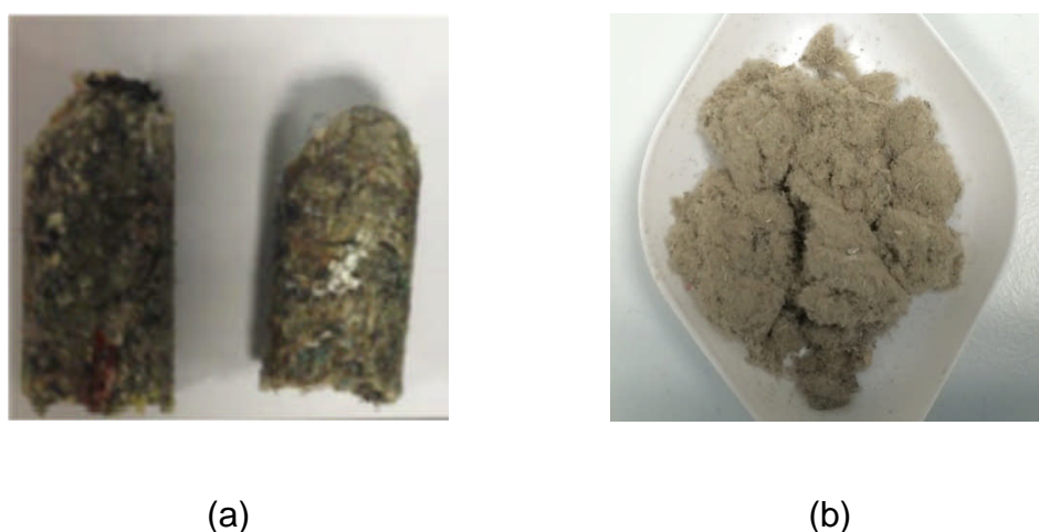
Figure 3.1.5 RDF sample (a) original pellets (b) shredded samples
