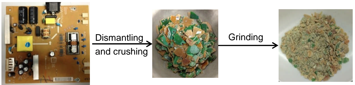
Figure 3.1.3 The printed circuit board extracted from desktop computer LCD monitors
