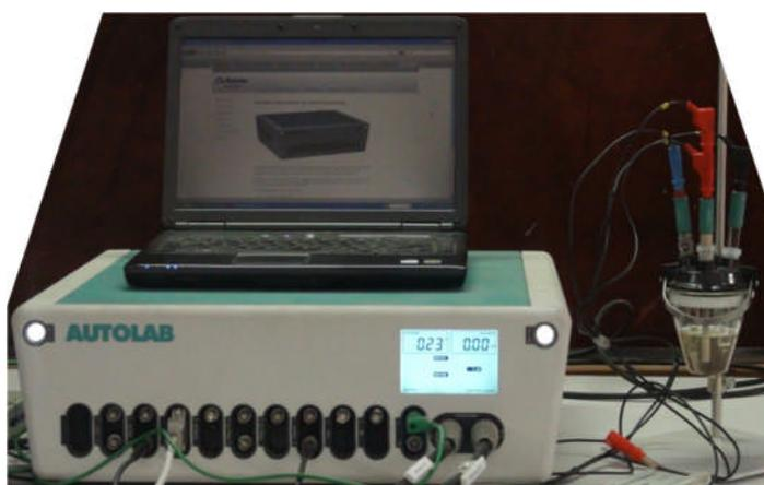
Figure 2.2: The first electrochemical set up: a photograph of fully assembled electrochemical cell connected to Autolab potentiostat.
