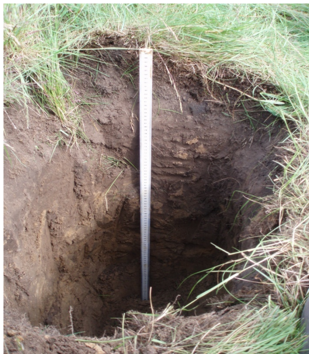
Plate 2.3: Typical acid grassland brown earth soil profile at Hob Moor. This is one of the acid brown earth profiles sampled for the ammonium absorption/desorption experiments described in detail in Chapter 5.
