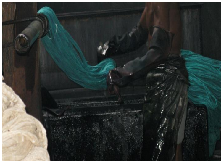
Fig 5.2 Dyeing of silk yarns in a cottage industry
