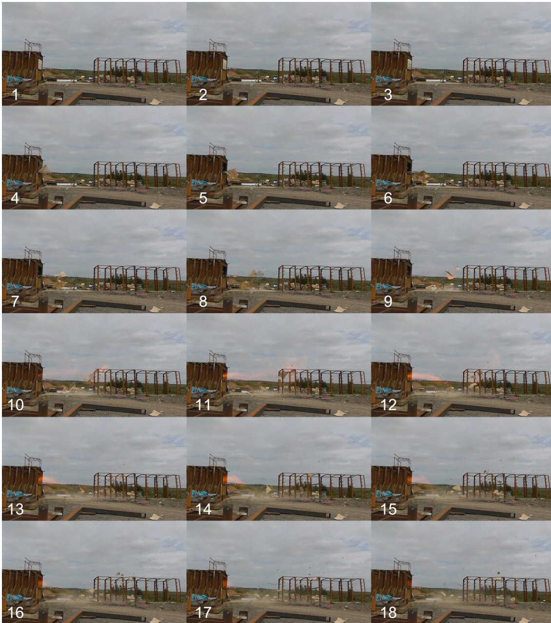
Figure 5-22 Photo sequence showing the later stages of a 10% methane/air explosion in an empty chamber
