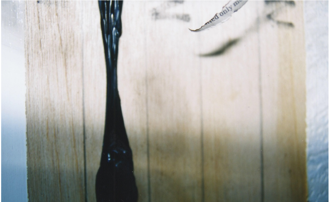
Figure 6-12 Thermal damage to polythene sheet (Spadeadam, Rig C)
