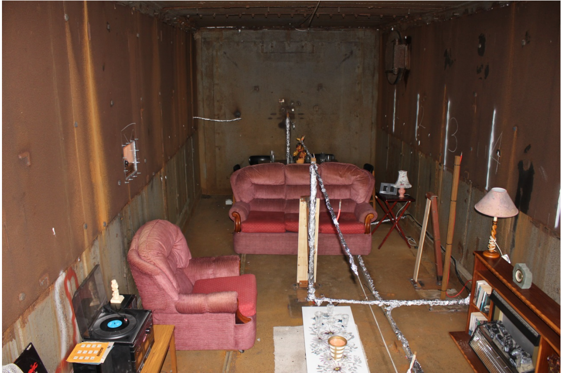
Figure 3-17 Typical furniture layout (Rig C)
