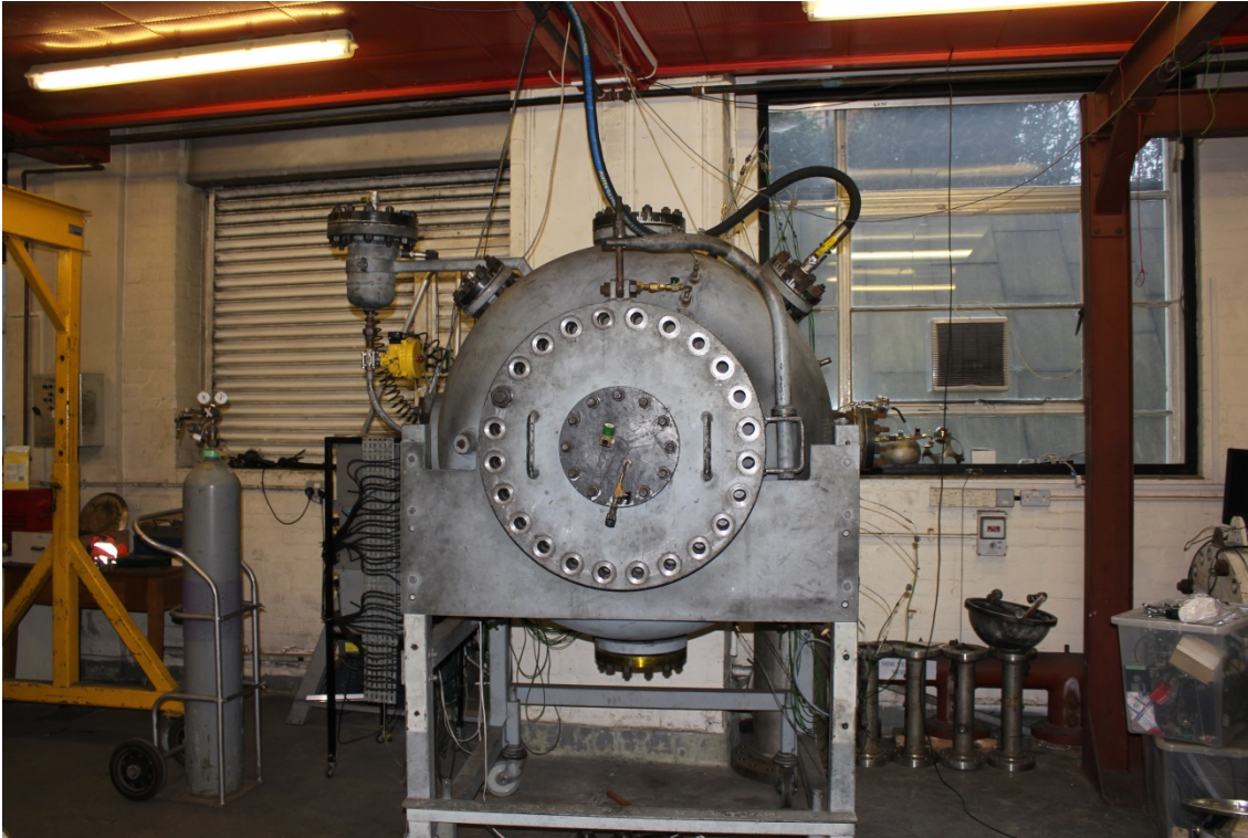
Figure 3-18 1m 3 explosion vessel – front elevation (Rig D)
