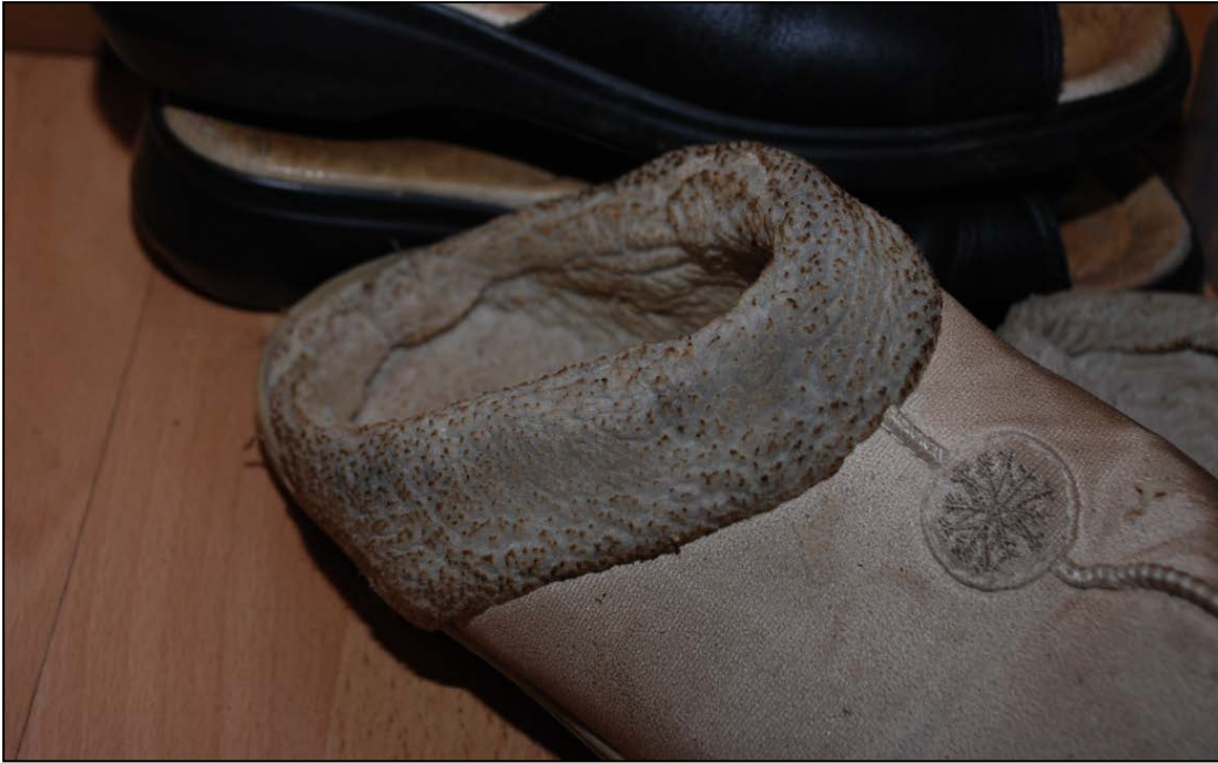
Figure 1-5 Evidence of thermal damage following a layered LPG explosion (photo taken by the author)
