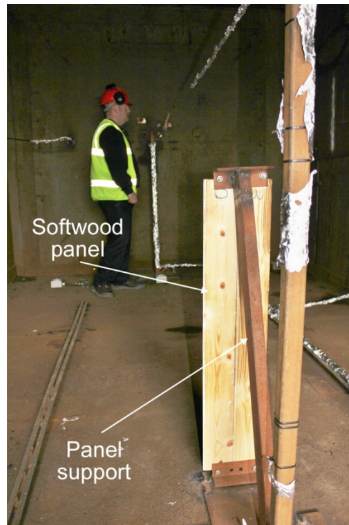
Figure 3-50 Softwood panel support (Rig C)
