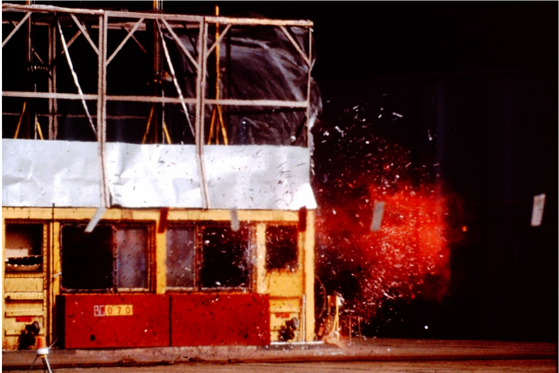
Figure 4-37 Failure of the right 4 mm single glass pane vent and secondary external explosion (taken from DNV GL archive)
