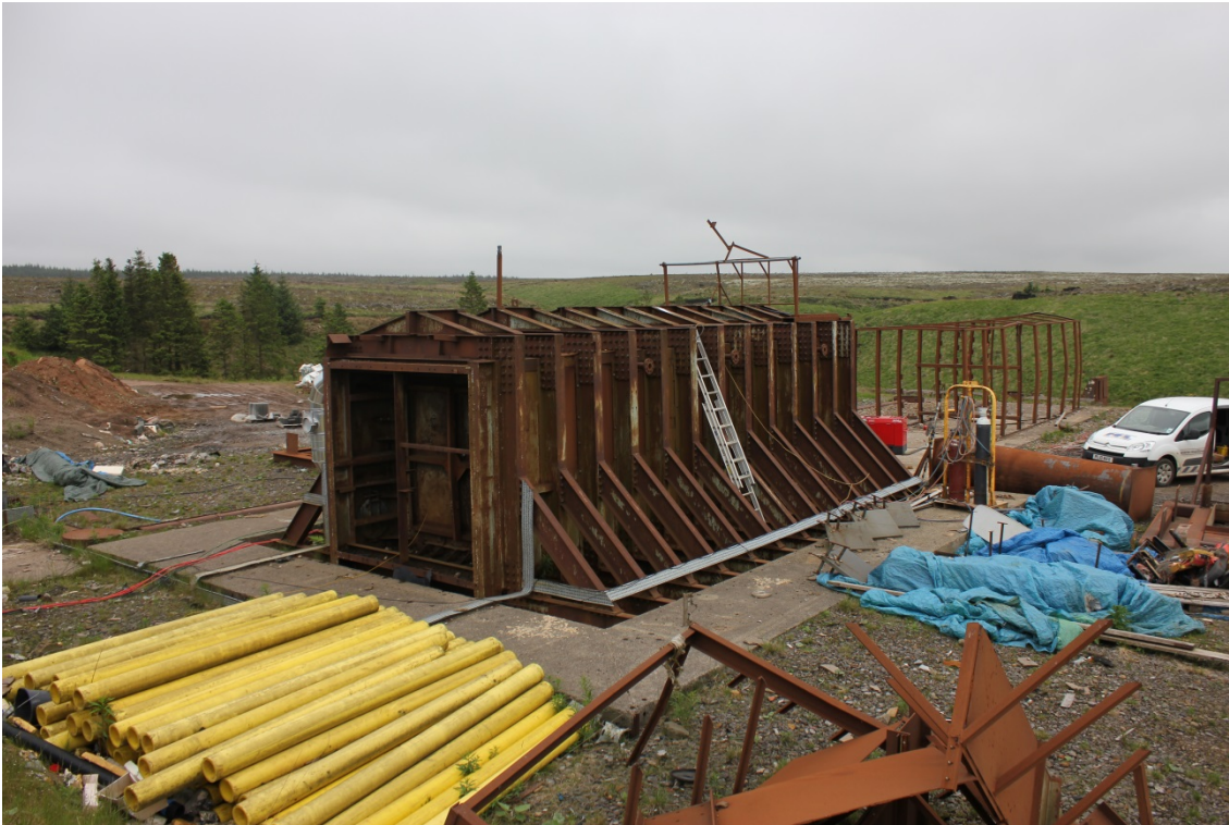
Figure 3-14 Spadeadam explosion chamber (Rig C)
