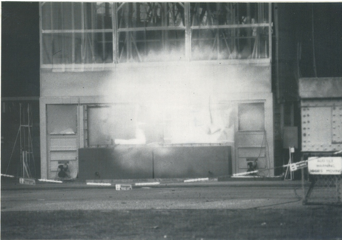
Figure 4-34 External explosion during test 85 (400 ms after ignition)
