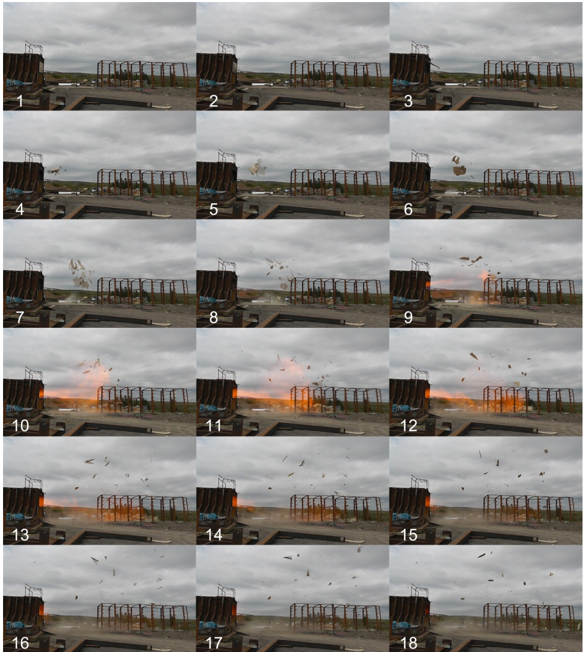
Figure 5-23 Photo sequence showing the later stages of a 12.5% methane/air explosion in an empty chamber
