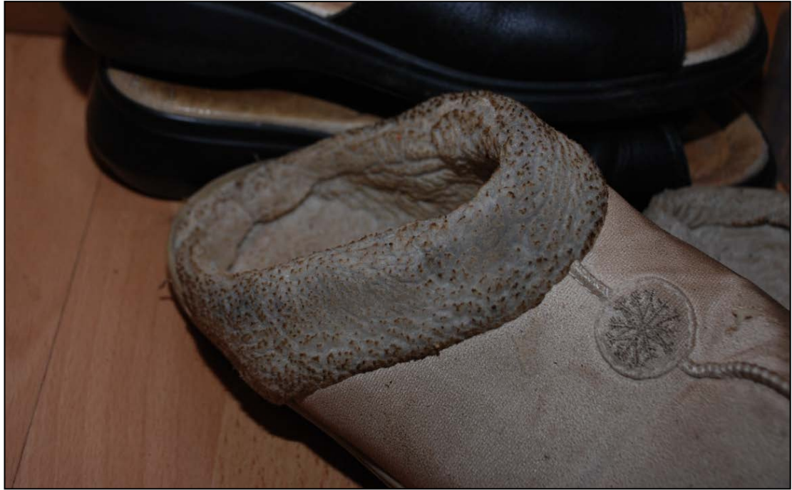
Figure 2-40 Evidence of thermal damage following a layered LPG explosion (photo taken by the author)
