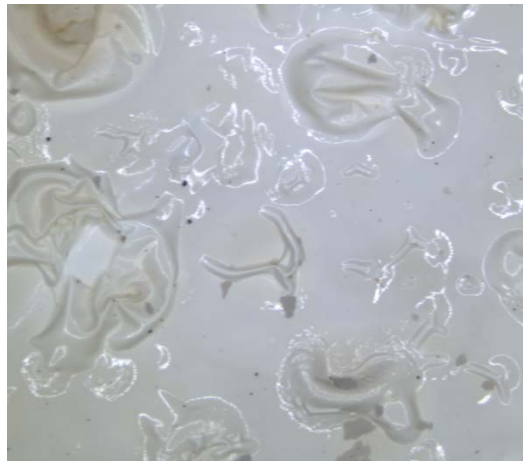
Figure 6-26 Stereo microscope image of a sample of painted wood (Spadeadam Rig C, test 2)
