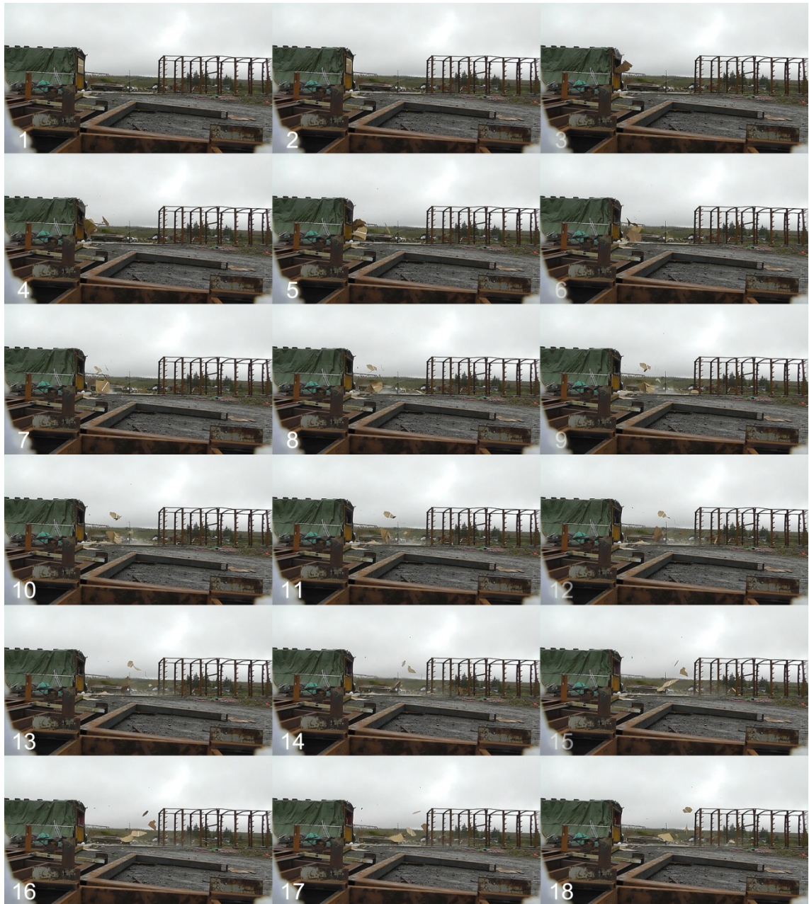
Figure 5-28 Photo sequence showing the later stages of a 7.5% methane/air explosion with 5% VB from furniture
