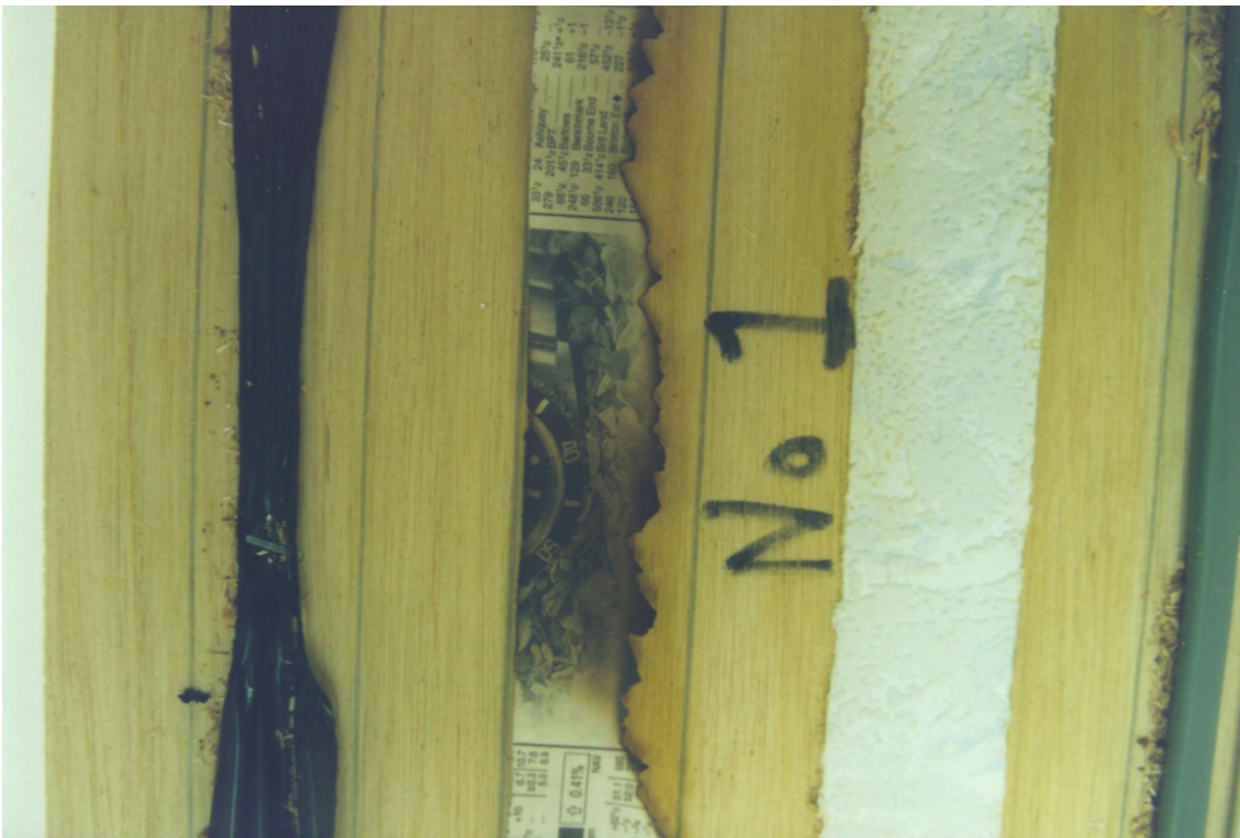
Figure 6-11 Thermal damage to newspaper (Spadeadam, Rig C)
