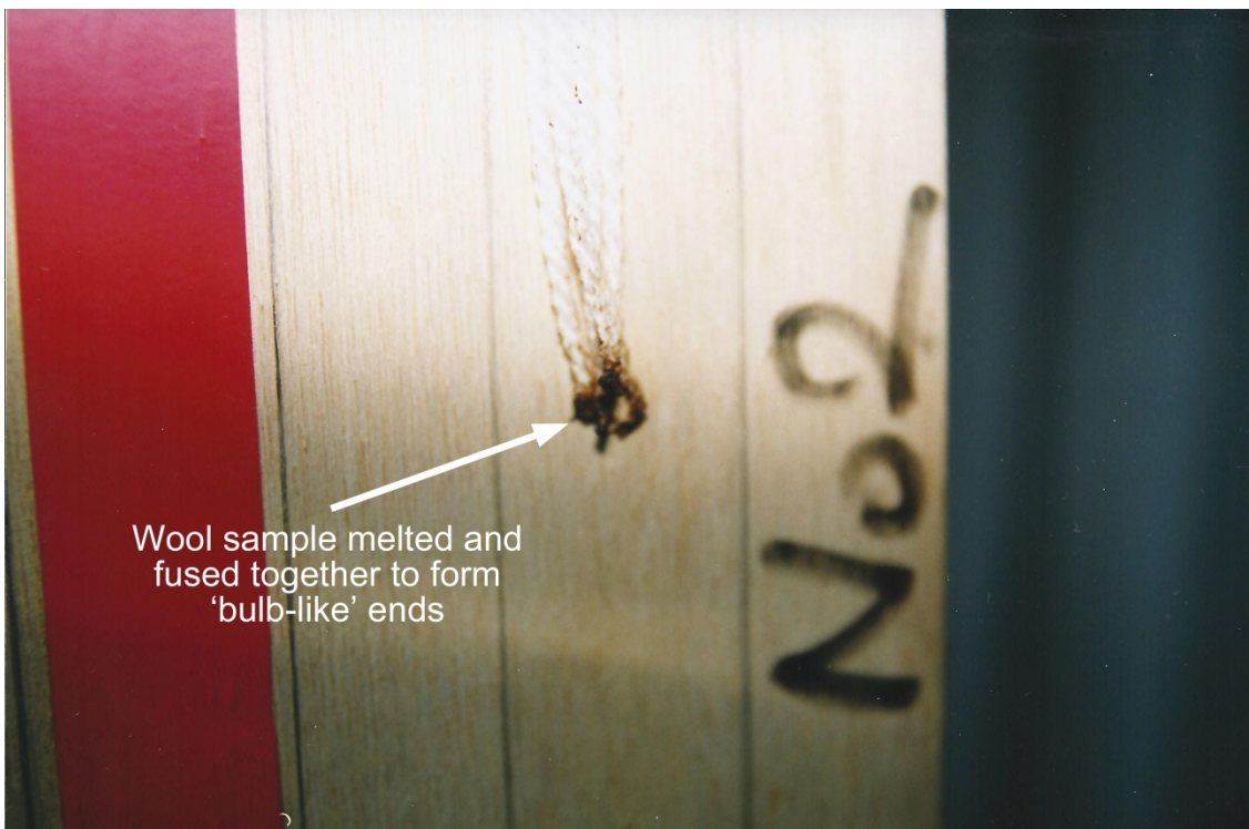
Figure 6-14 Thermal damage to cotton wool (Spadeadam, Rig C)
