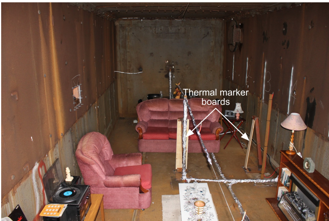
Figure 3-51 Location of thermal marker stands prior to explosion test (Rig C)
