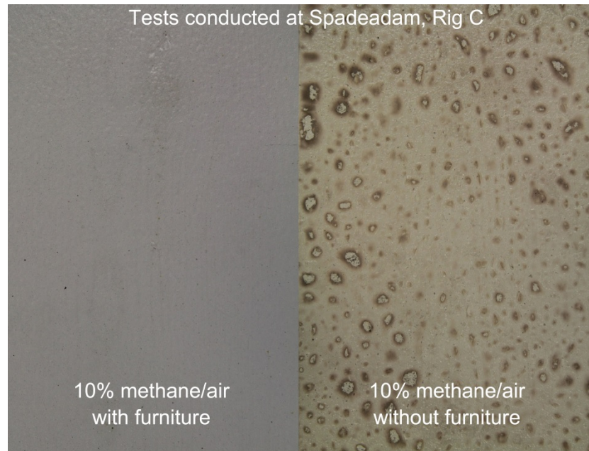
Figure 6-23 The effect of flame speed on thermal damage
