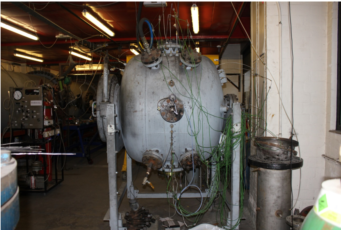
Figure 3-19 1m 3 explosion vessel – side elevation (Rig D)
