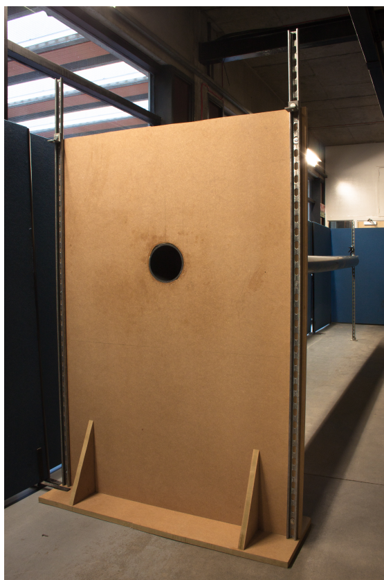
Figure 3.1: A photograph of the open flanged pipe used for the experiments.
