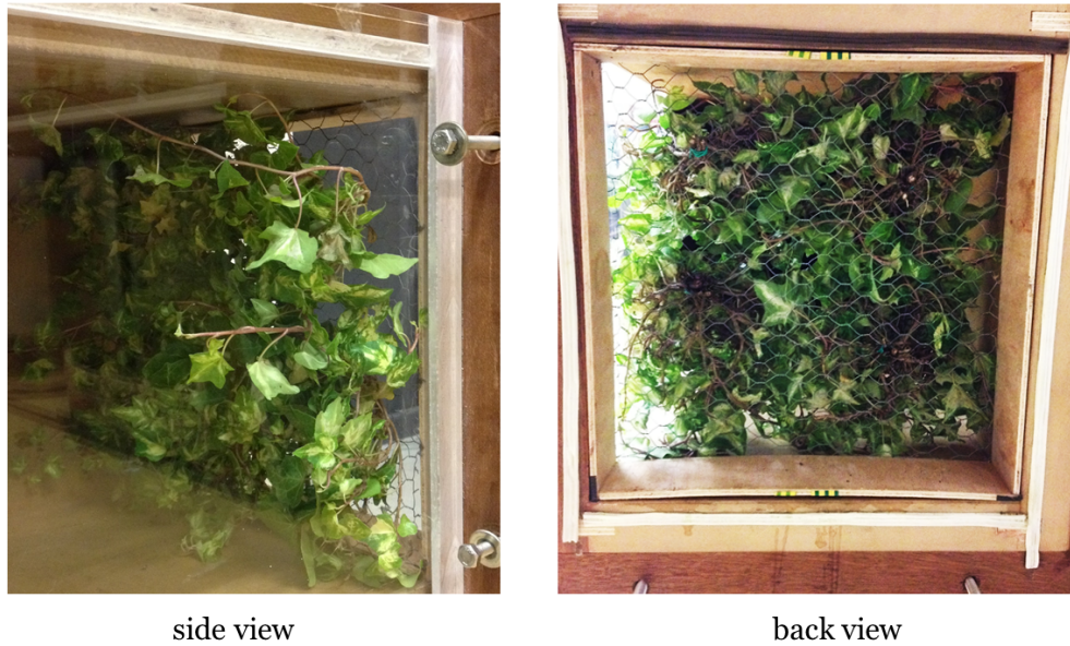
Figure 6.2: The wooden frame used for holding the living plants parallel to the bottom of the tube. On the left: side view; on the right: back view.
