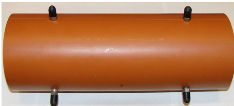
Figure 4.2: A photograph of the coaxial cylinder used as a blockage.
