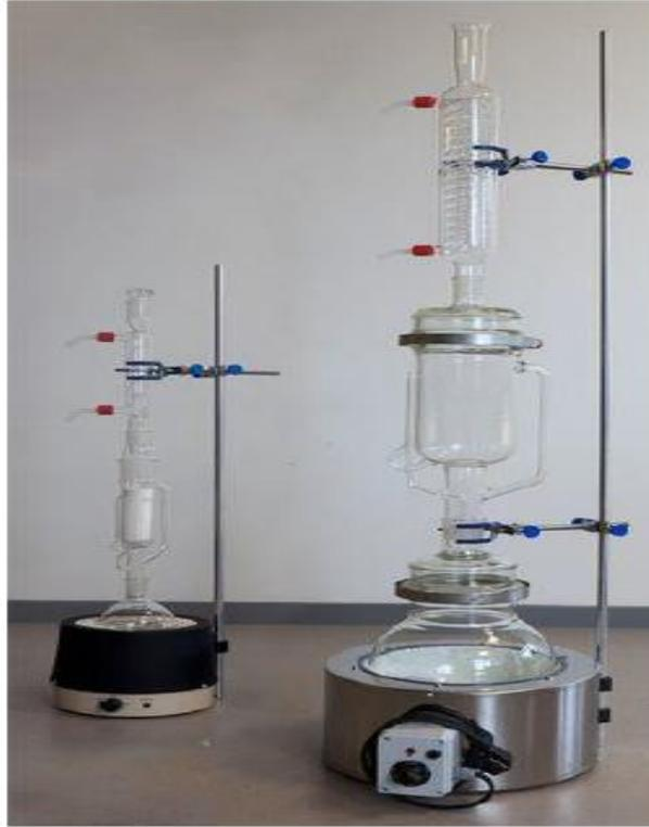
*Figure 3.7 The Dean stark distillation apparatus for sample cleaning (taken from vinci Tech catalogue).*
