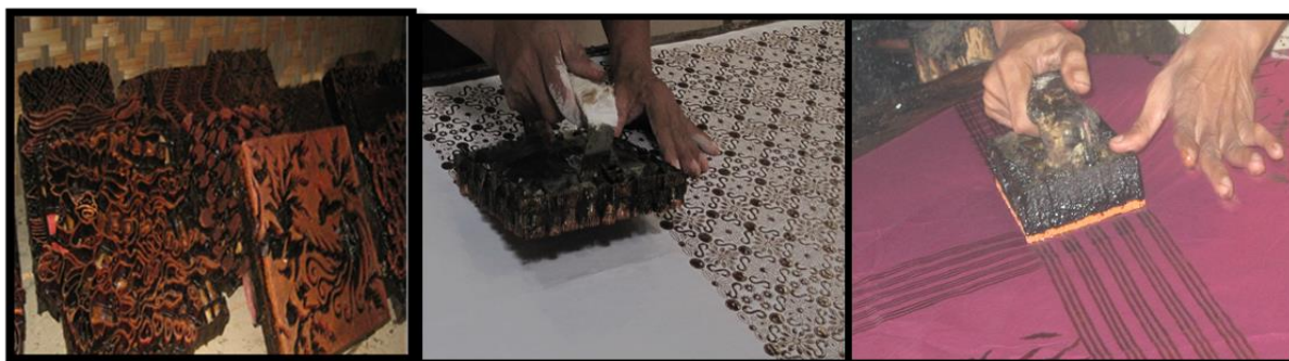
Figure 1.6 Hand-stamping batik process
