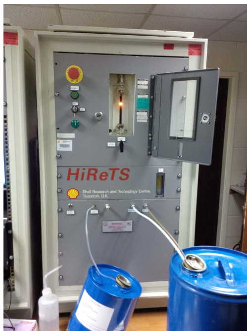
Figure 5.1: Photograph of the HiReTS Thermal Stability Test Rig.
