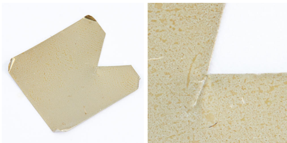
(a) Uniform brown coating on foil with a part unsplit for SEM and EDX analysis.
