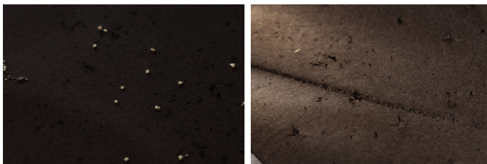
(c) Tiny spherical deposits on a metal foil placed in 2,2,4-trimethylpentane with dibutylsulfide with a dark carbon like coating. (d) Tiny filamentous deposits on a dark coating on a metal foil placed in 2,2,4-trimethylpentane with p-xylene and dibutylsulfide.
