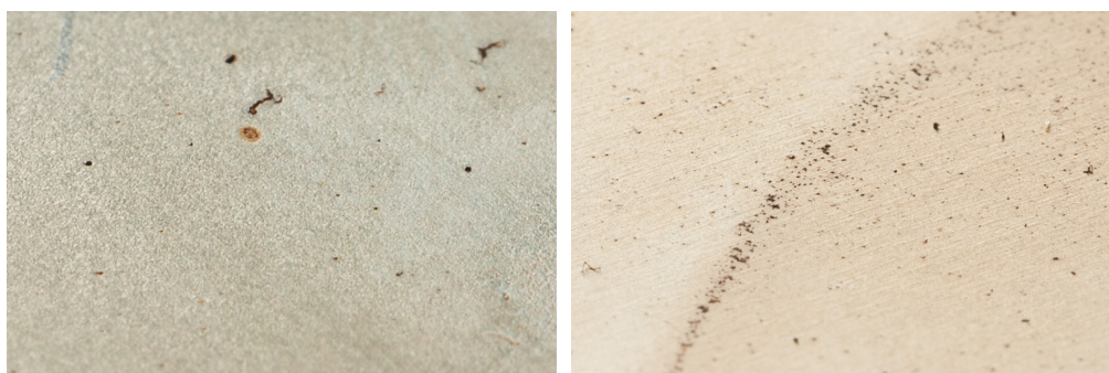
(a) Tiny filamentous deposits with a “powder-like looking coating” on a metal foil placed in 2,2,4-trimethylpentane and dibutylsulfide. (b) Tiny particulate deposits on a metal foil placed in 2,2,4-trimethylpentane with p-xylene and dibutylsulfide.
