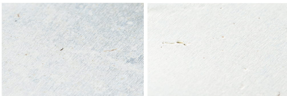
(a) Tiny filamentous deposits between yellowish spots on a metal foil placed in dodecane and dibutylsulfide. (b) A small amount of tiny particulates on what is a liquid film coating on a metal foil placed in dodecane with p-xylene and dibutylsulfide.
