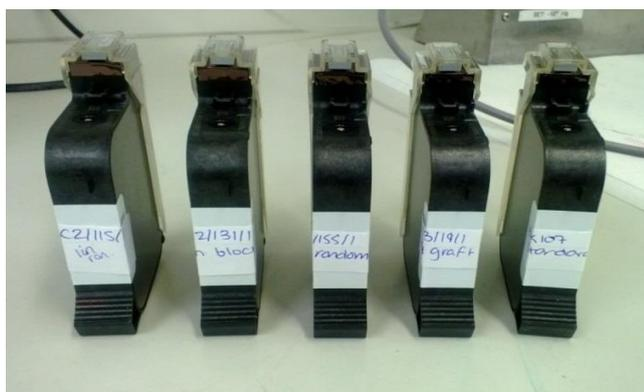
**Figure 8.6.** Cartridges filled with BK107 ink formulations for use on the G Series printer
