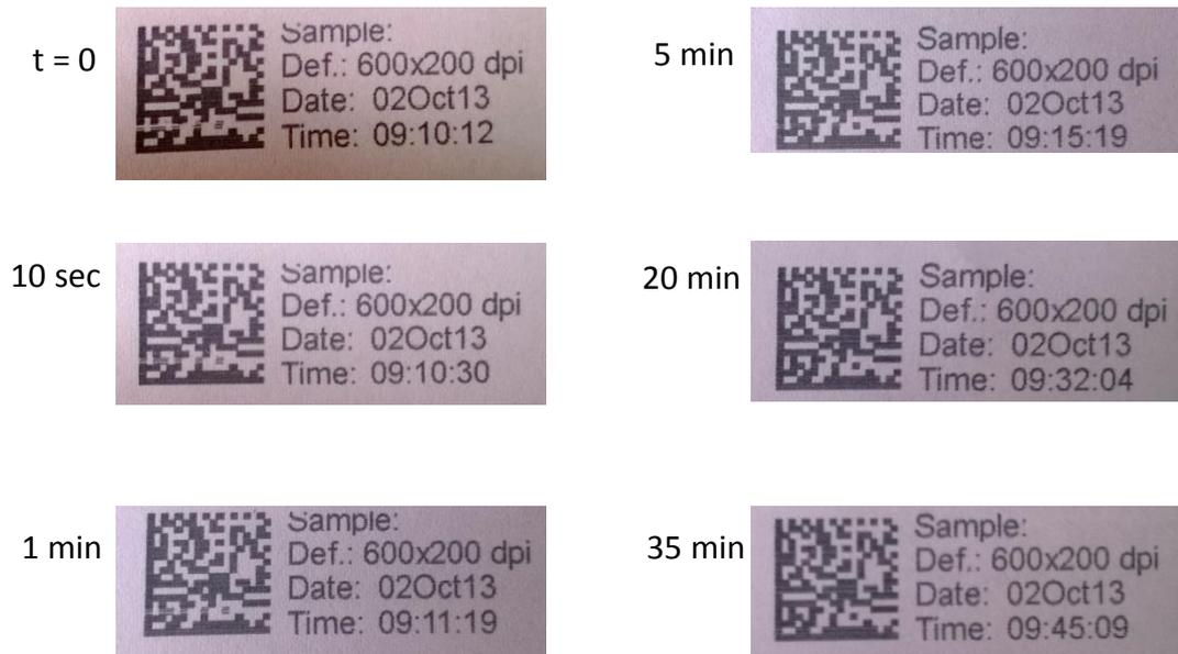
**Figure 8.9.** Prints of sample barcode using BK107 ink with 1.0% HB P(BMA-*co*-AA) copolymer at time intervals  $t = 0, 10 \text{ s}, 1 \text{ min}, 5 \text{ min}, 20 \text{ min},$  and 35 min to study decap time
