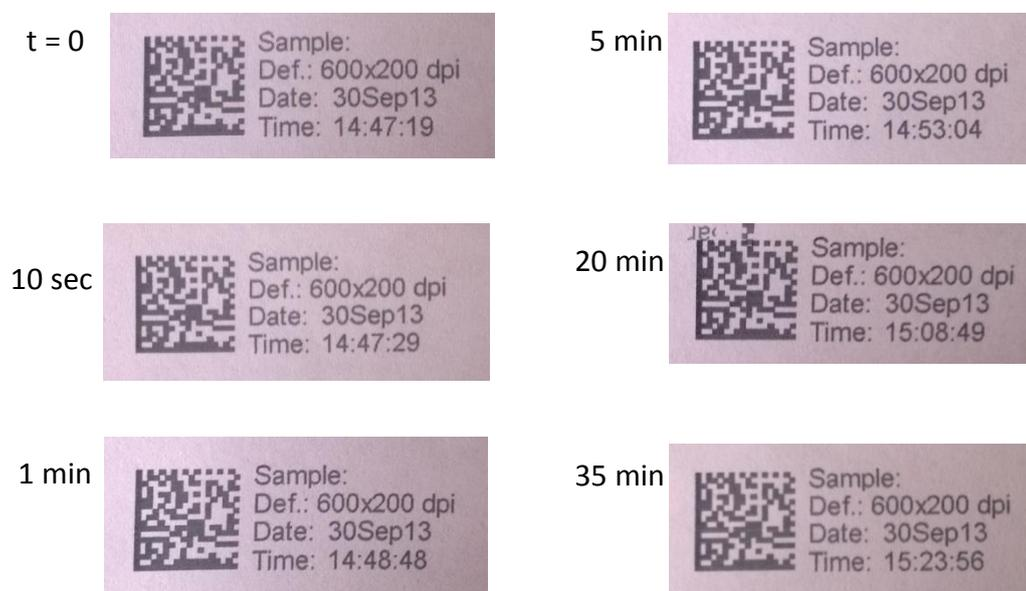
**Figure 8.7.** Prints of sample barcode using BK107 ink with 0.5% HB P(BMA-*co*-AA) copolymer at time intervals:  $t = 0$ , 10 s, 1 min, 5 min, 20 min, and 35 min to study decap time
