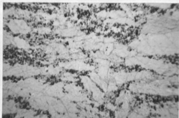
JG814(3) Carbonatite, Kerimasi. Ord. light. X 28. The dark veins contain magnetite, forsterite, and spinel.
