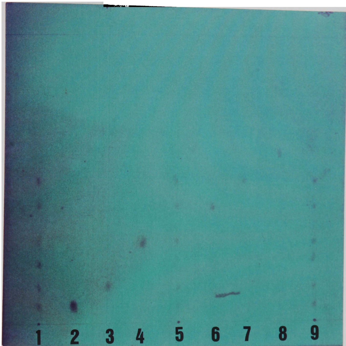
Figure 4.10 :- T.L.C. of Monocarboxylic Acids formed during the Thermal Oxidation of MXD,6 at 180°C.
