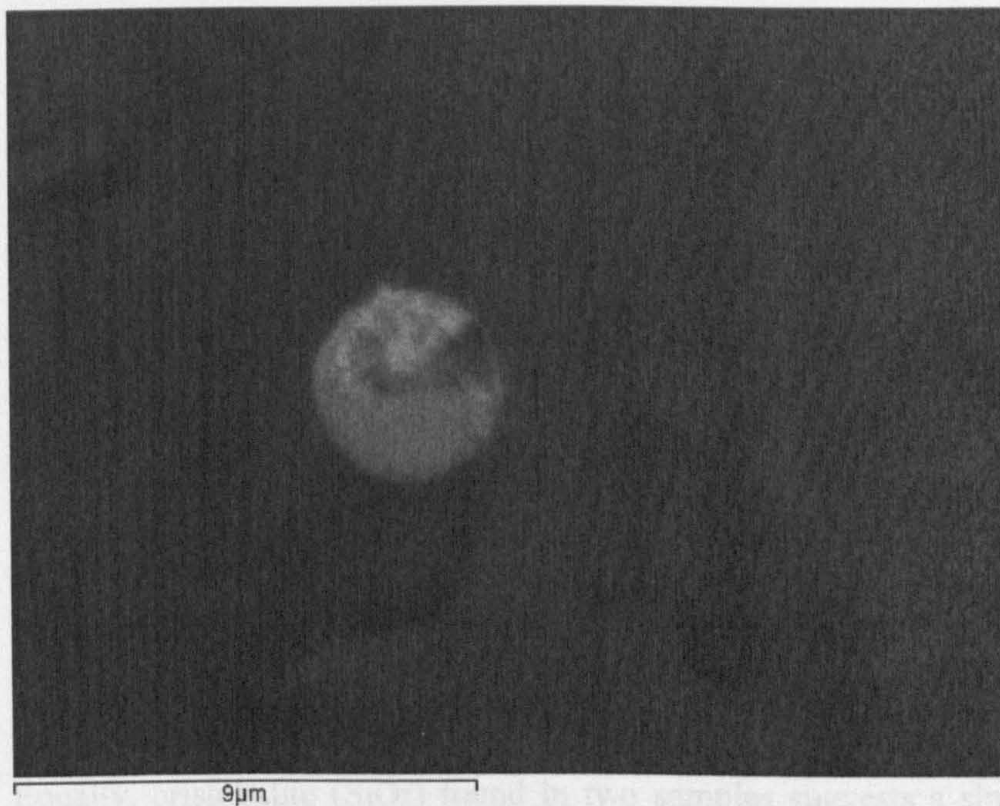
Figure 6.14 MAK02 : glassy matrix (black) and spheroid speiss inclusion consisting of Fe: 6.72%, Pb: 22.2%, Cu: 1.43%, As: 10.74%, Sb: 24% (SEM photomicrograph)
