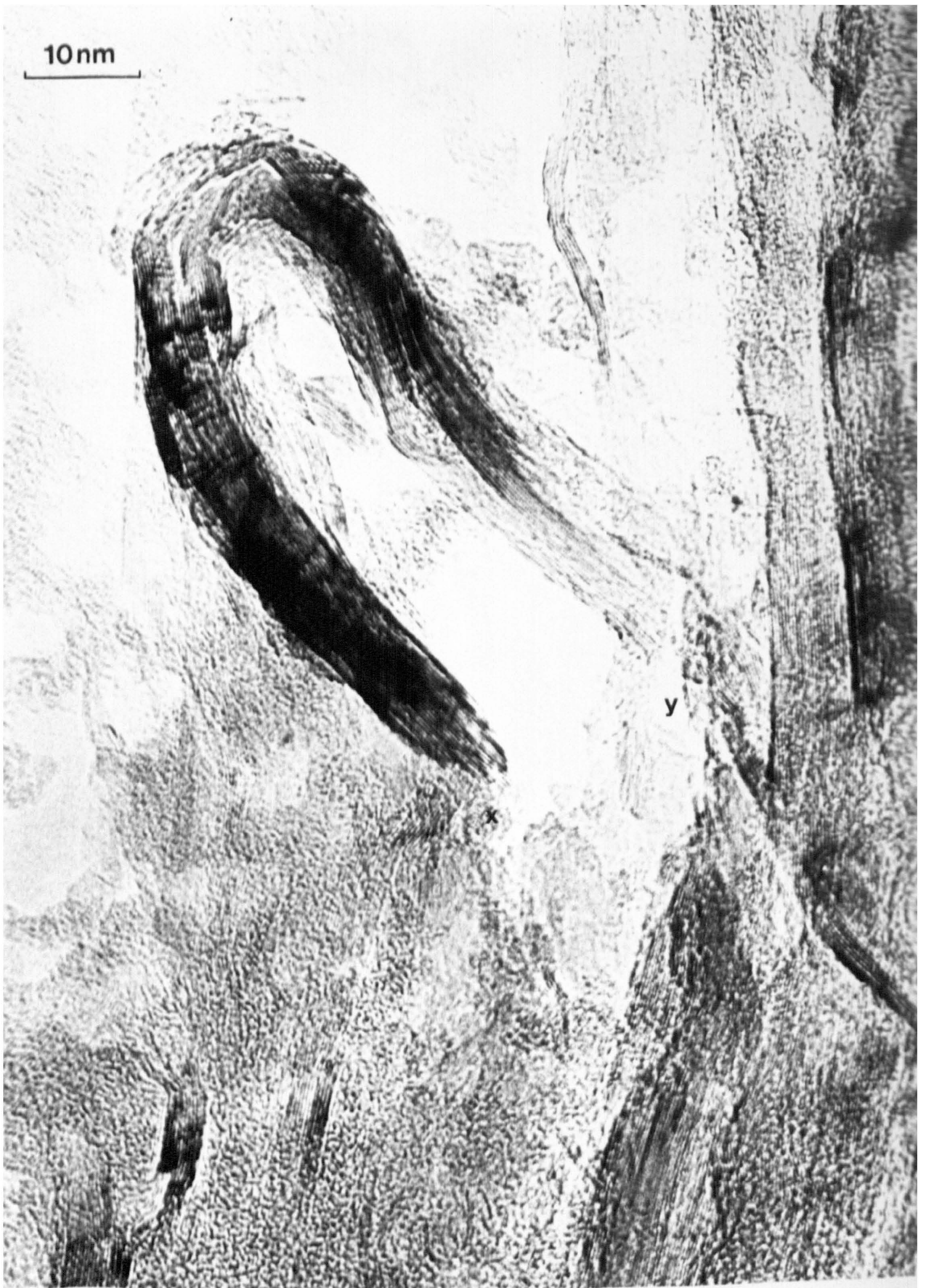
Plate XII. Lattice-resolution image of a 'hair-pin' flaw in the skin structure of specimen C2500.
