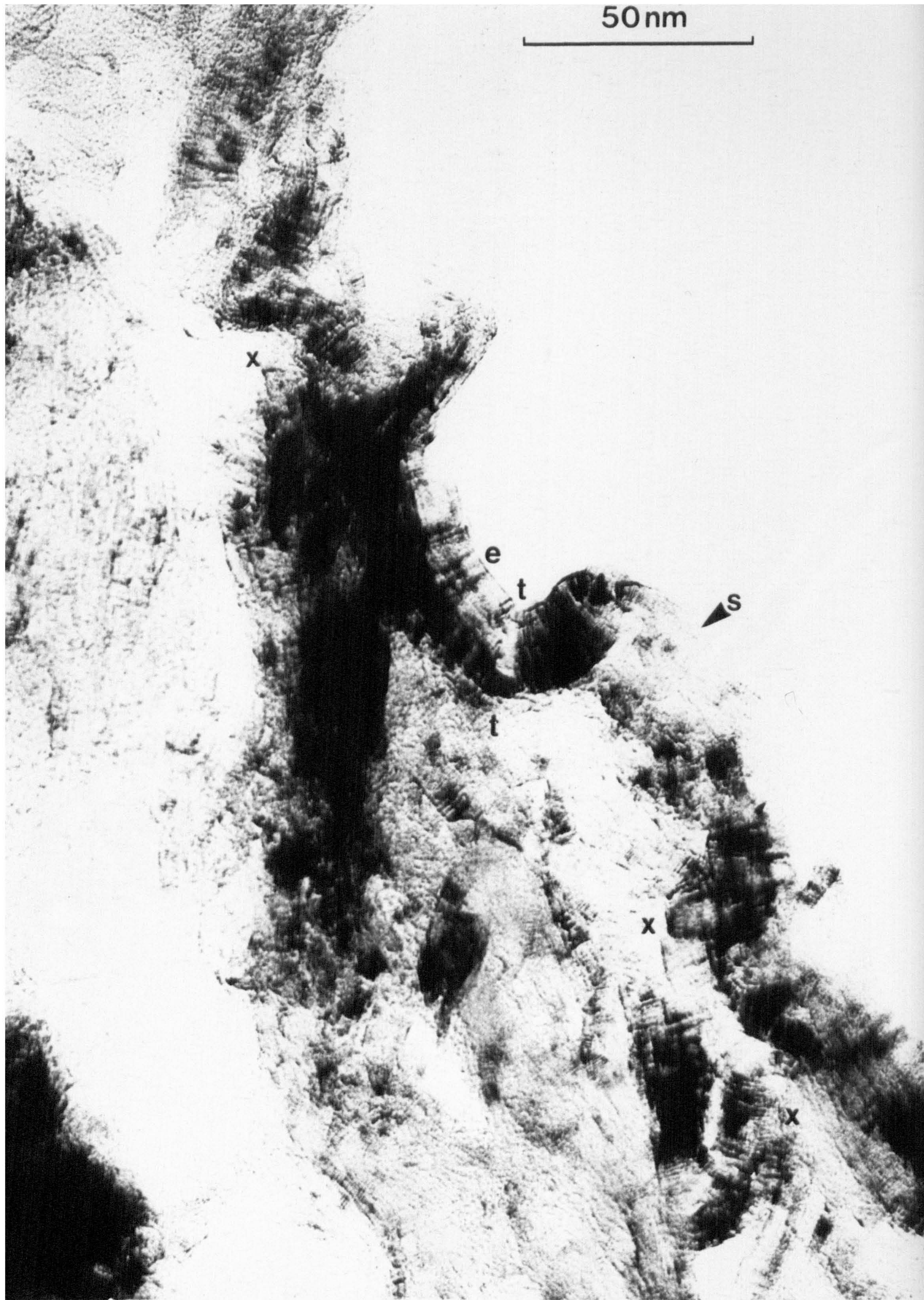
Plate L. Lattice-resolution image of the skin structure in a transverse section of specimen S2500.
