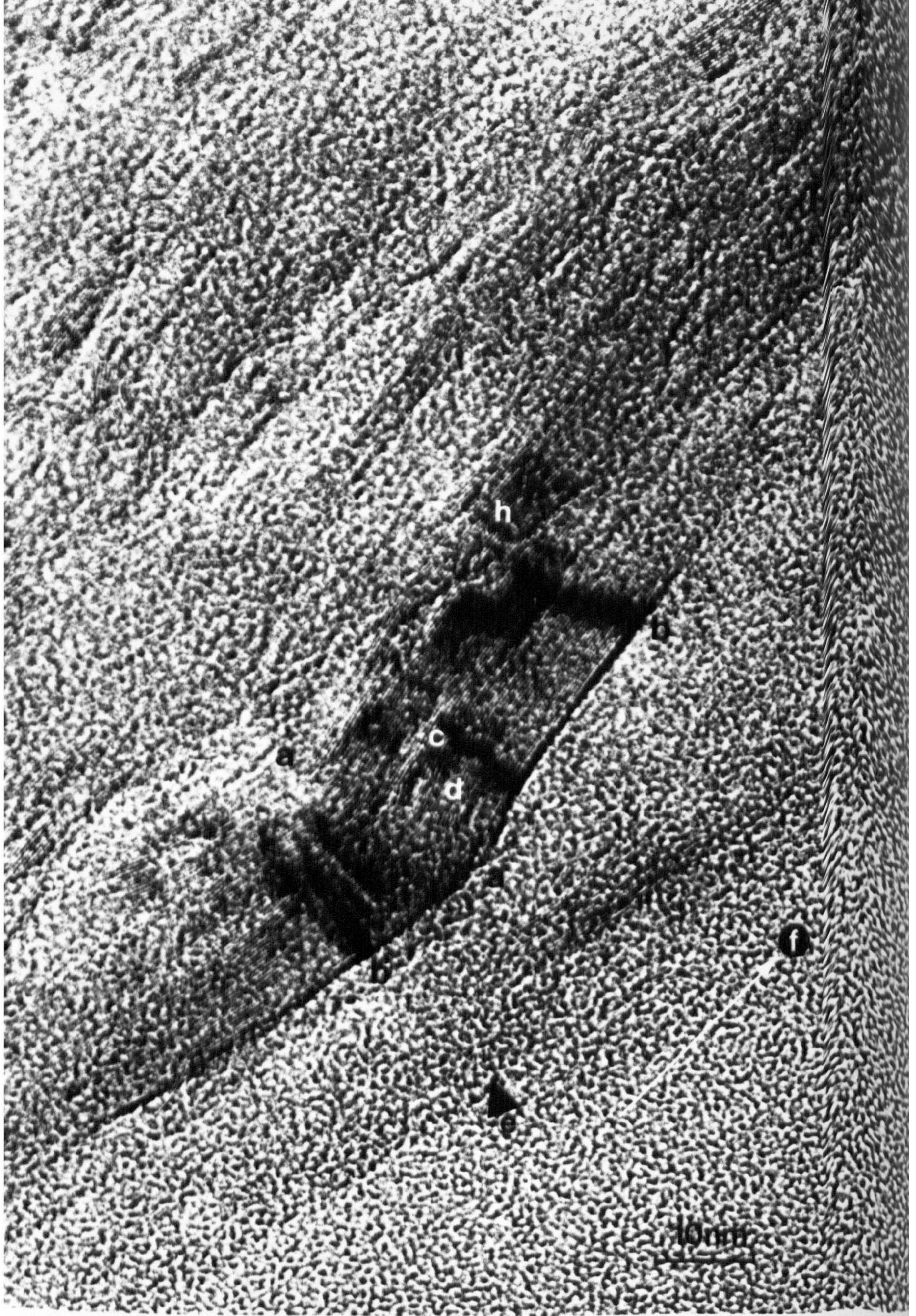
Plate XVII. Lattice-resolution image of 'knee-shaped' flaw in the skin structure of specimen F2500.
