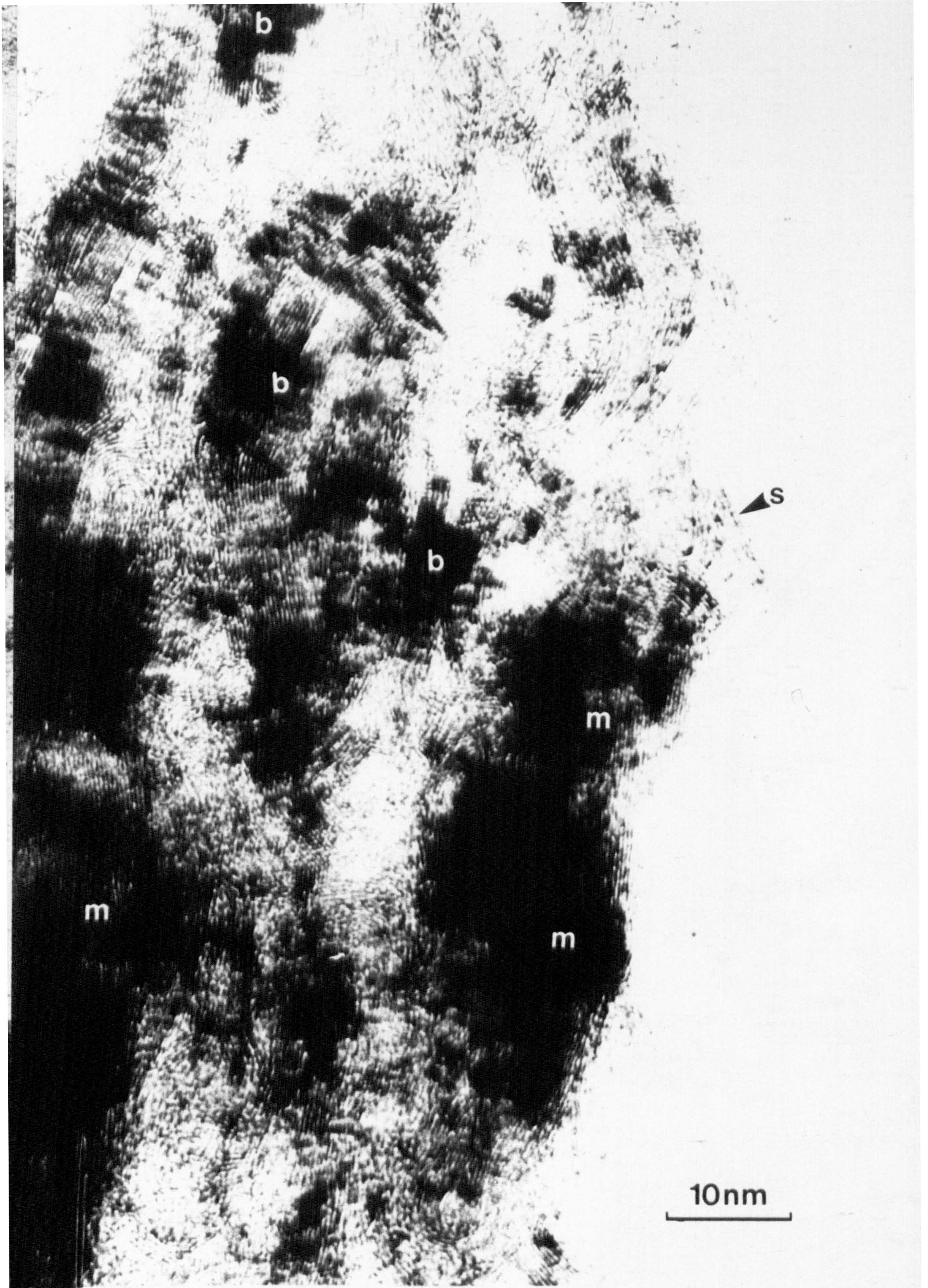
Plate LI. Lattice-resolution image of the skin structure in a transverse section of specimen R2500.
