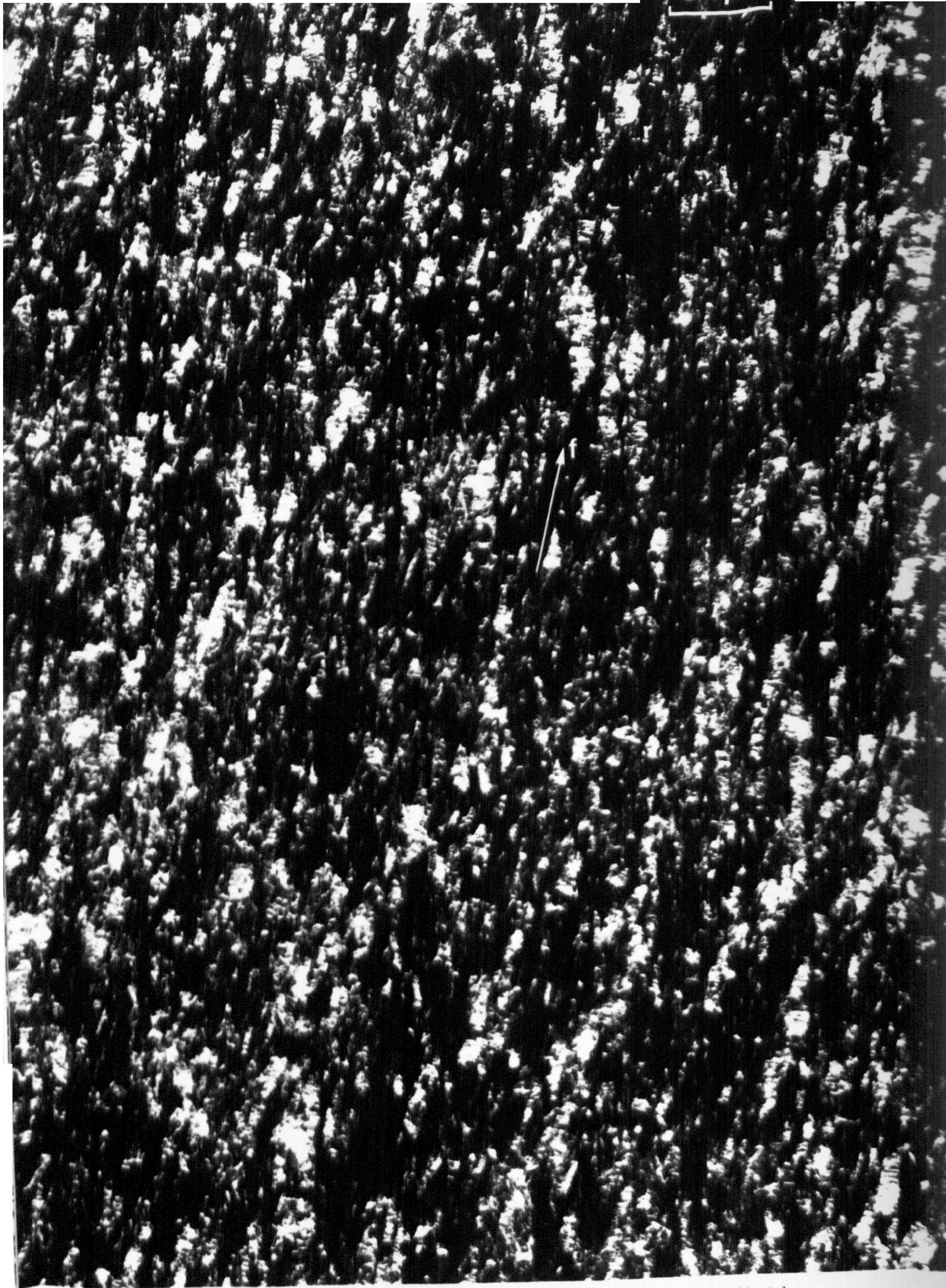
Plate VI. Intermediate-magnification (002) dark-field image of the core structure of specimen F2500.
