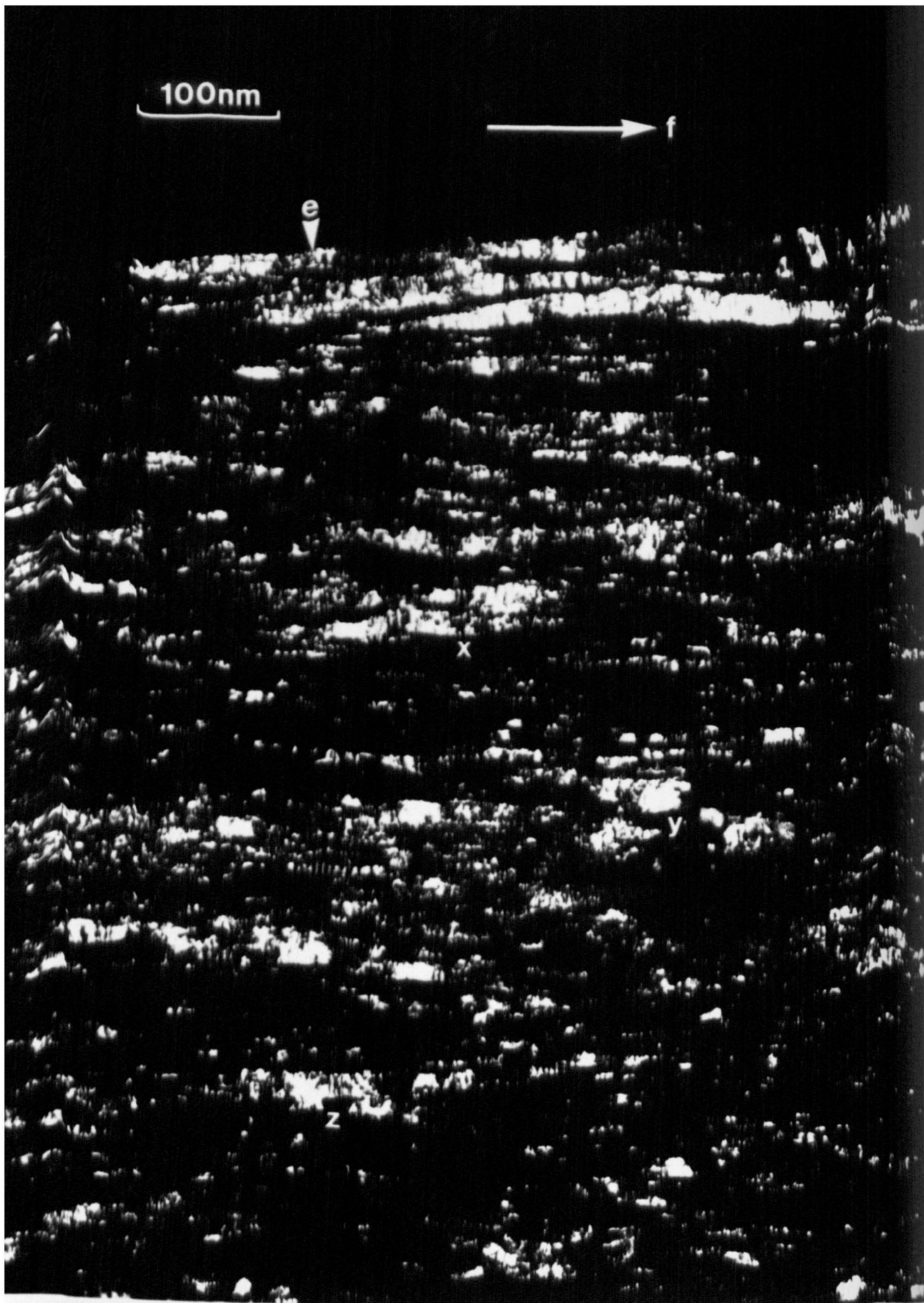
Plate XXXVI. Intermediate-magnification (002) dark-field image of the skin structure of specimen L2500.
