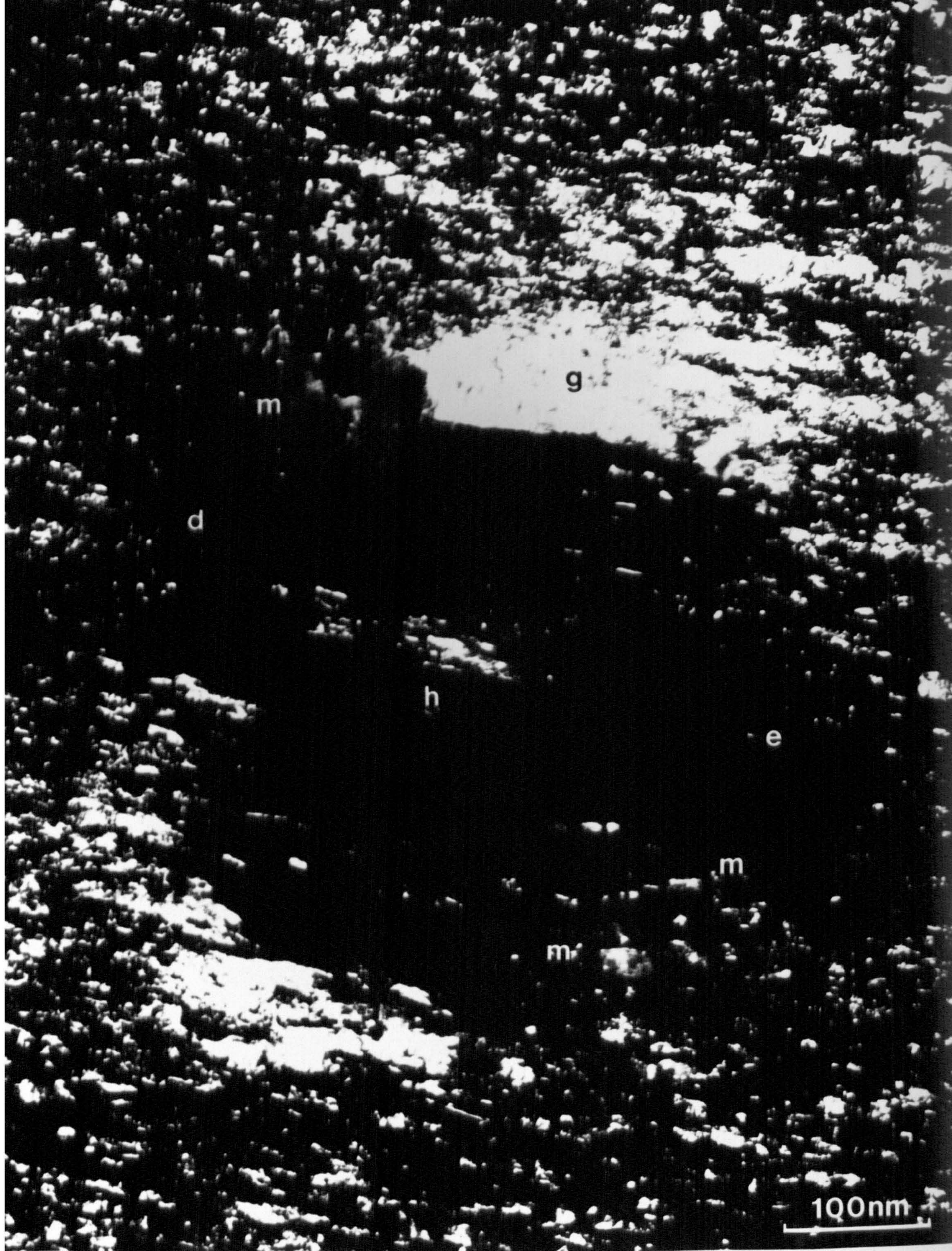
Plate XXIV. Intermediate-magnification (002) dark-field image of an internal void in specimen J2500.
