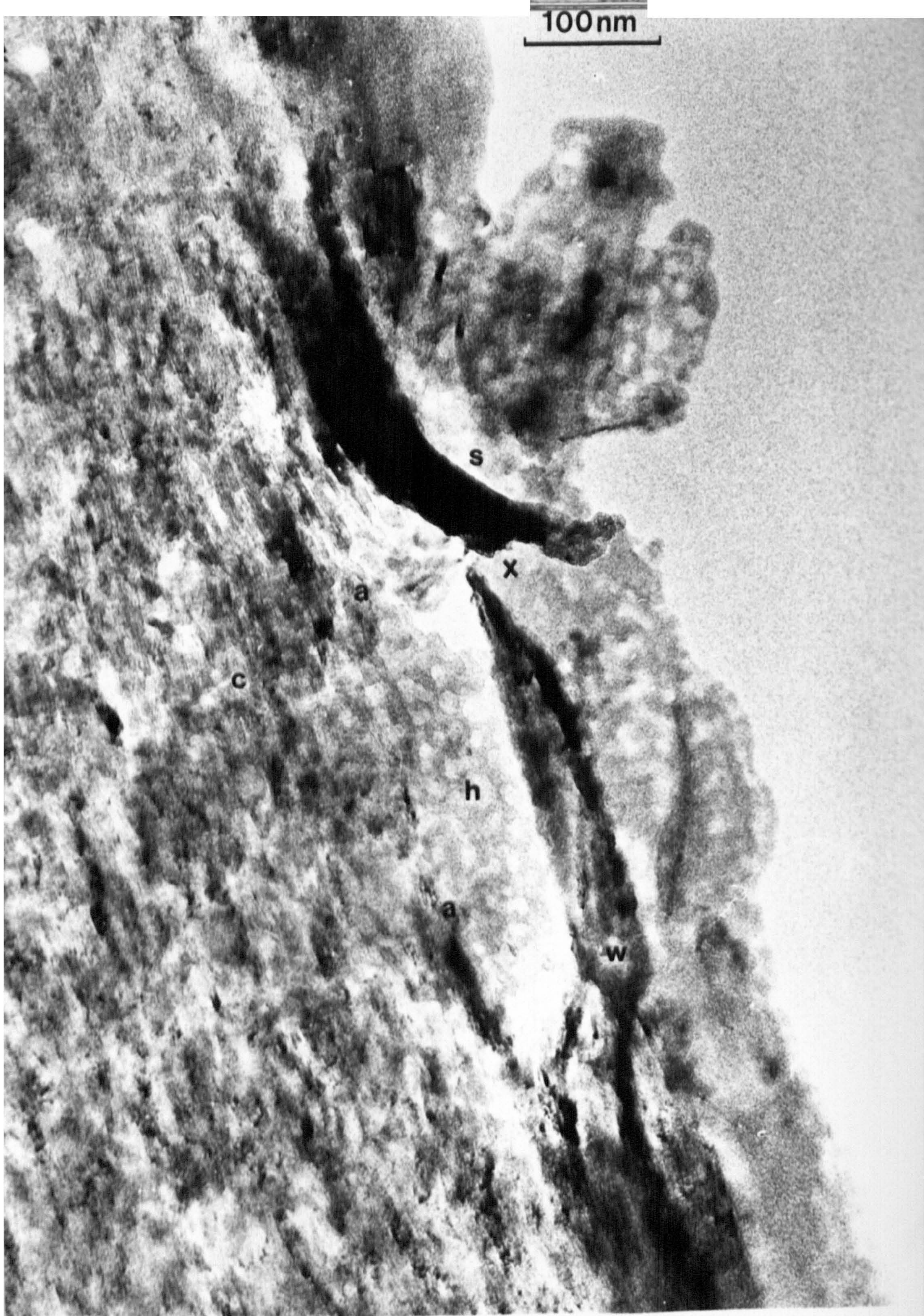
Plate XI. Intermediate-magnification bright-field image of a gross flaw in the skin structure of specimen B2500.
