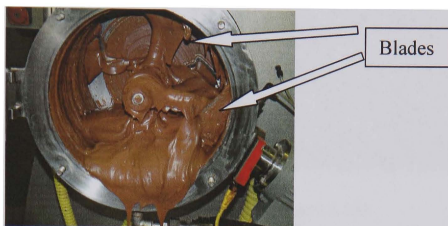
Figure 1.12: Picture of the inner view of the conche. Blades are fully coated by chocolate.
