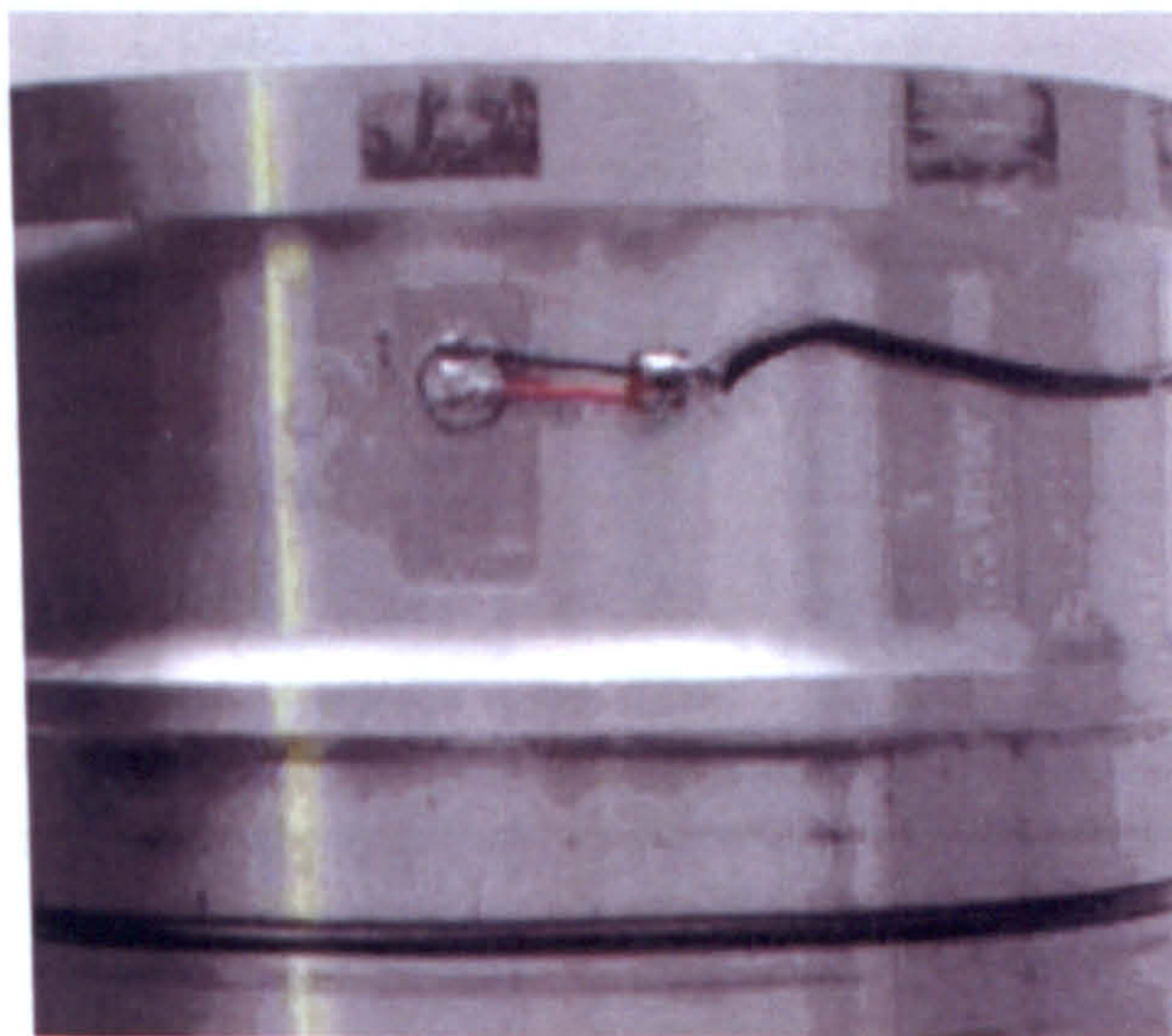
Figure 9.2: Photograph of the cylinder liner with the ultrasonic transducer bonded to the outer face.
