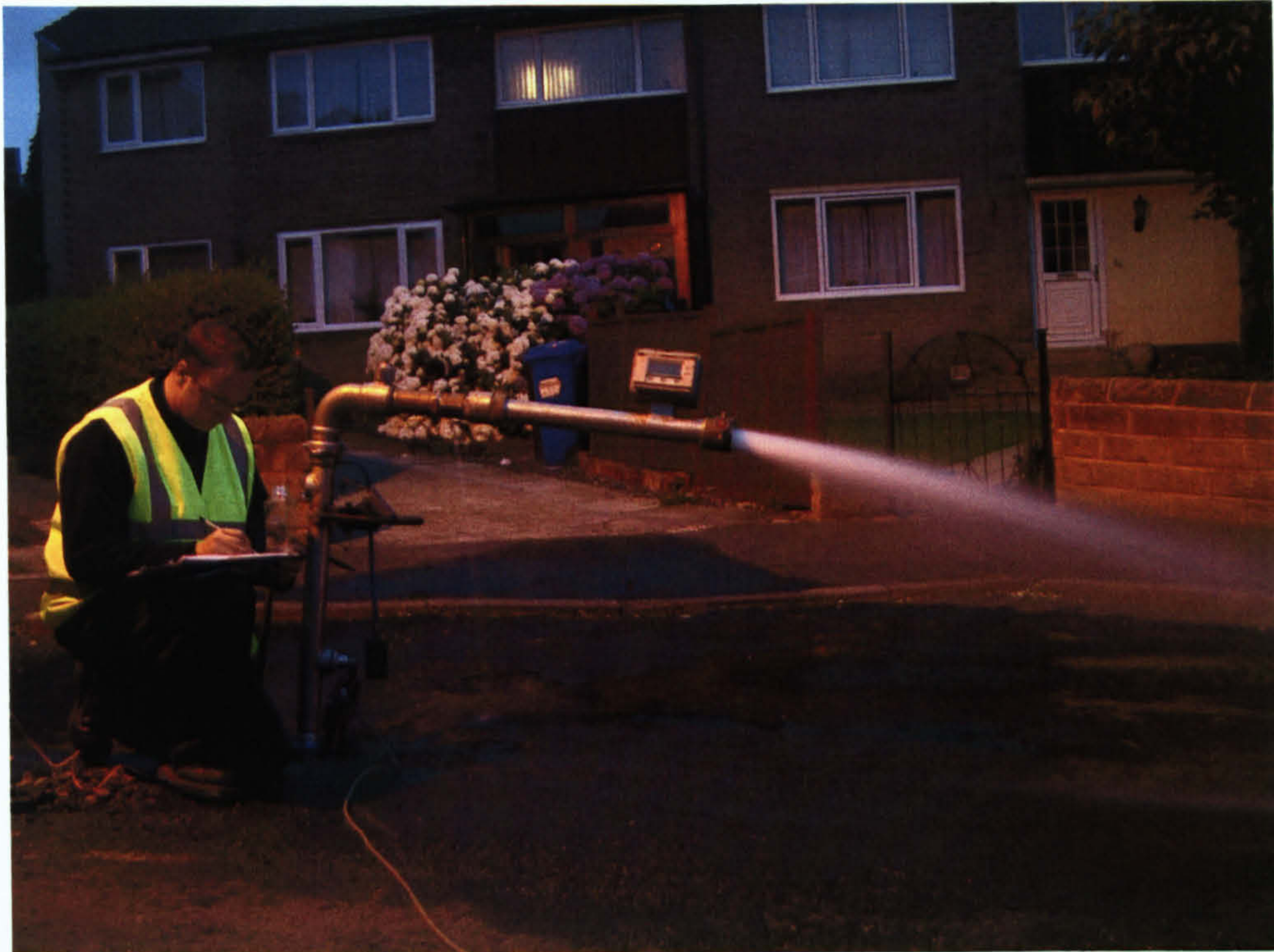
Figure 42 Flushing setup normal operation.
