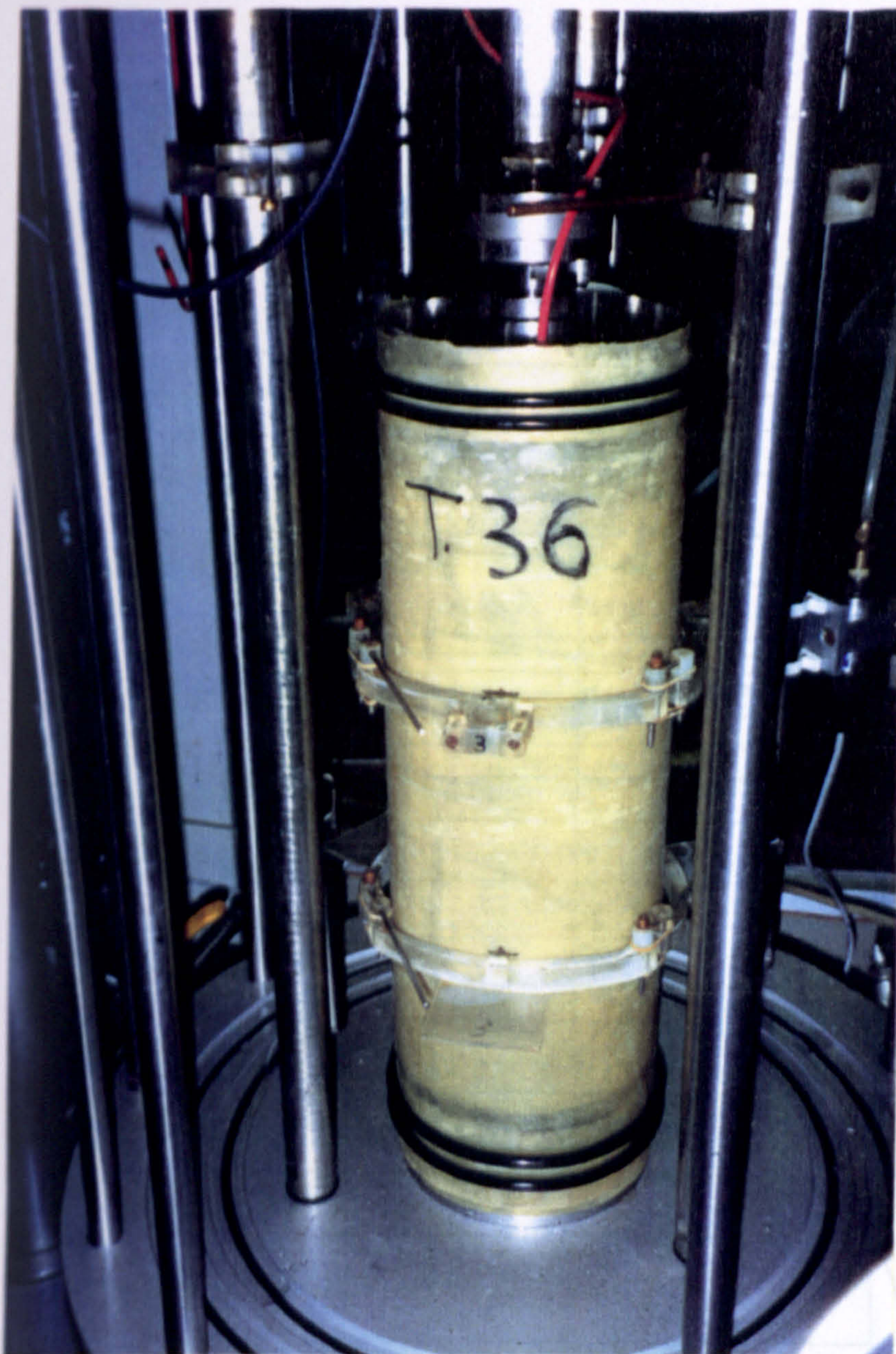
Plate 6.12 (Left)- The specimen after fixing the mounting system of the axial LVDTs
