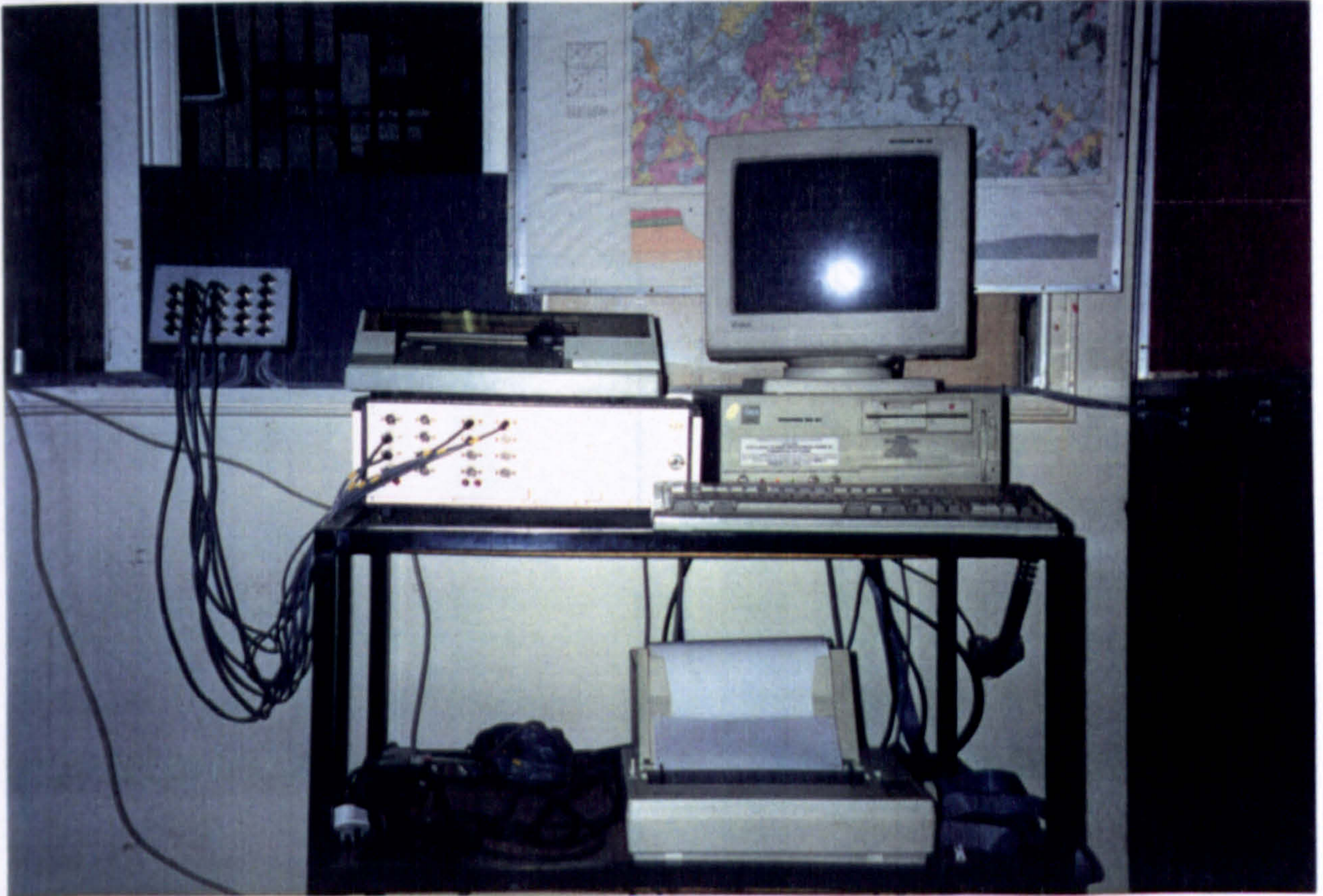
Plate 4.5- Logging system of the conventional triaxial cell
