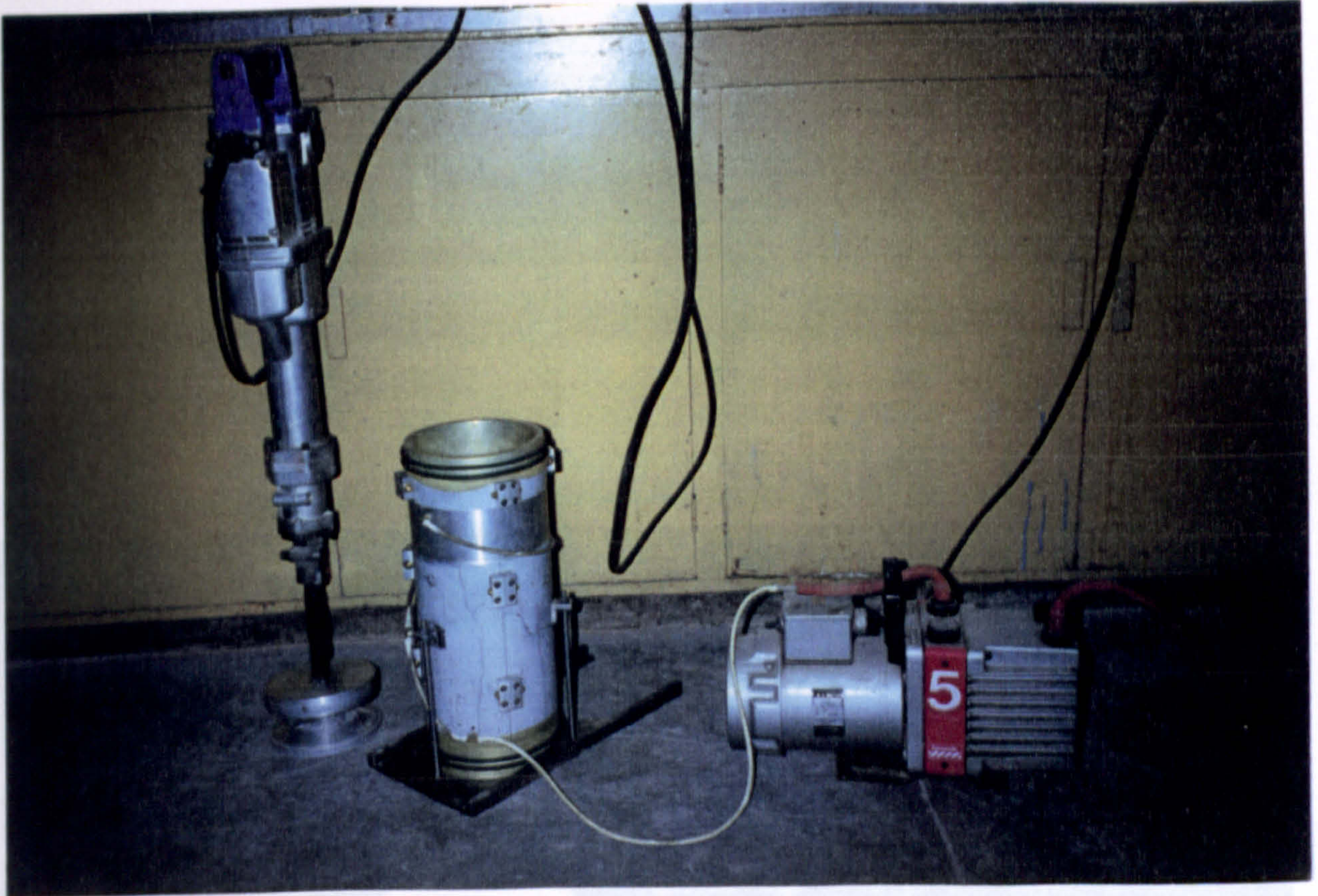
Plate 6.3- Kango compaction hammer, mould and vacuum pump
