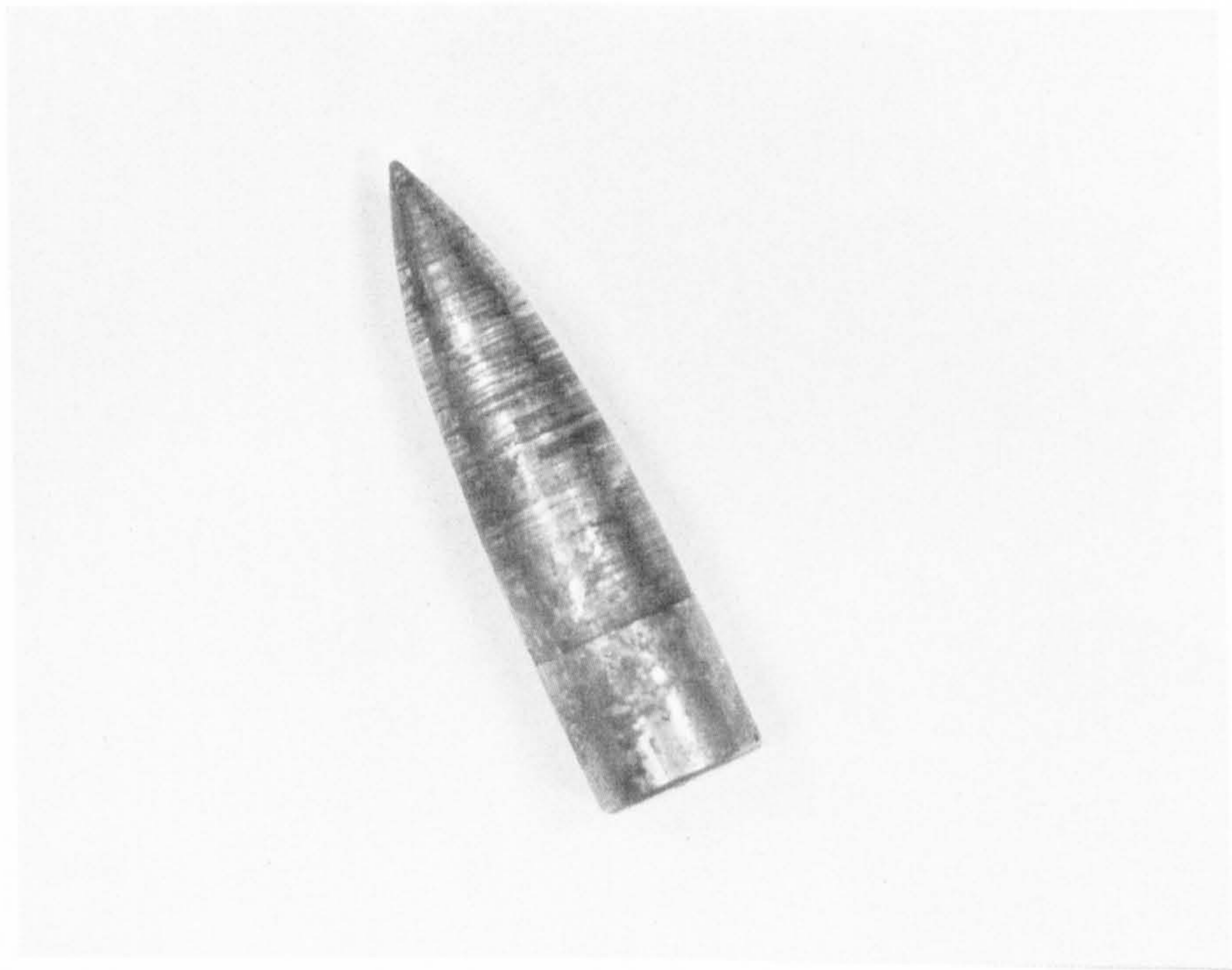
Figure 4.17 Hardened steel core after impact into mild steel target
